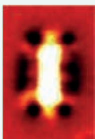
Near-field image of a rectangle graphene nanoresonator.
