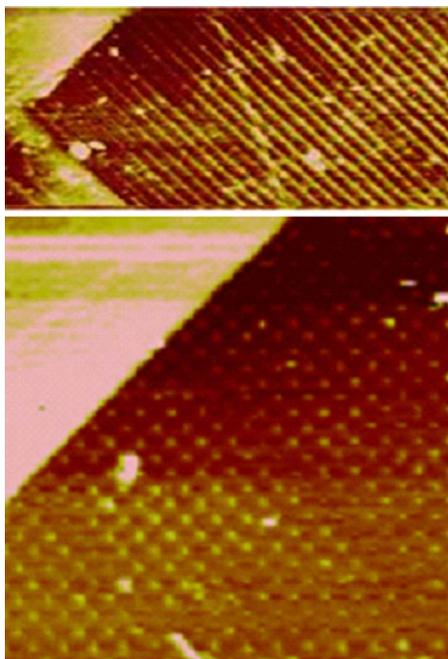
FIG. 11. (Color online) Large-area MFM images of the 2D patterned FePt films obtained by ion irradiation (dose= $1 \times 10^{14}$  ions/cm<sup>2</sup>) showing contrast from hard/soft regions: (a)  $1 \mu\text{m}$  stripes, (b)  $1 \mu\text{m}$ -diameter dots array. The signal in the dark-irradiated regions is due to background noise.
