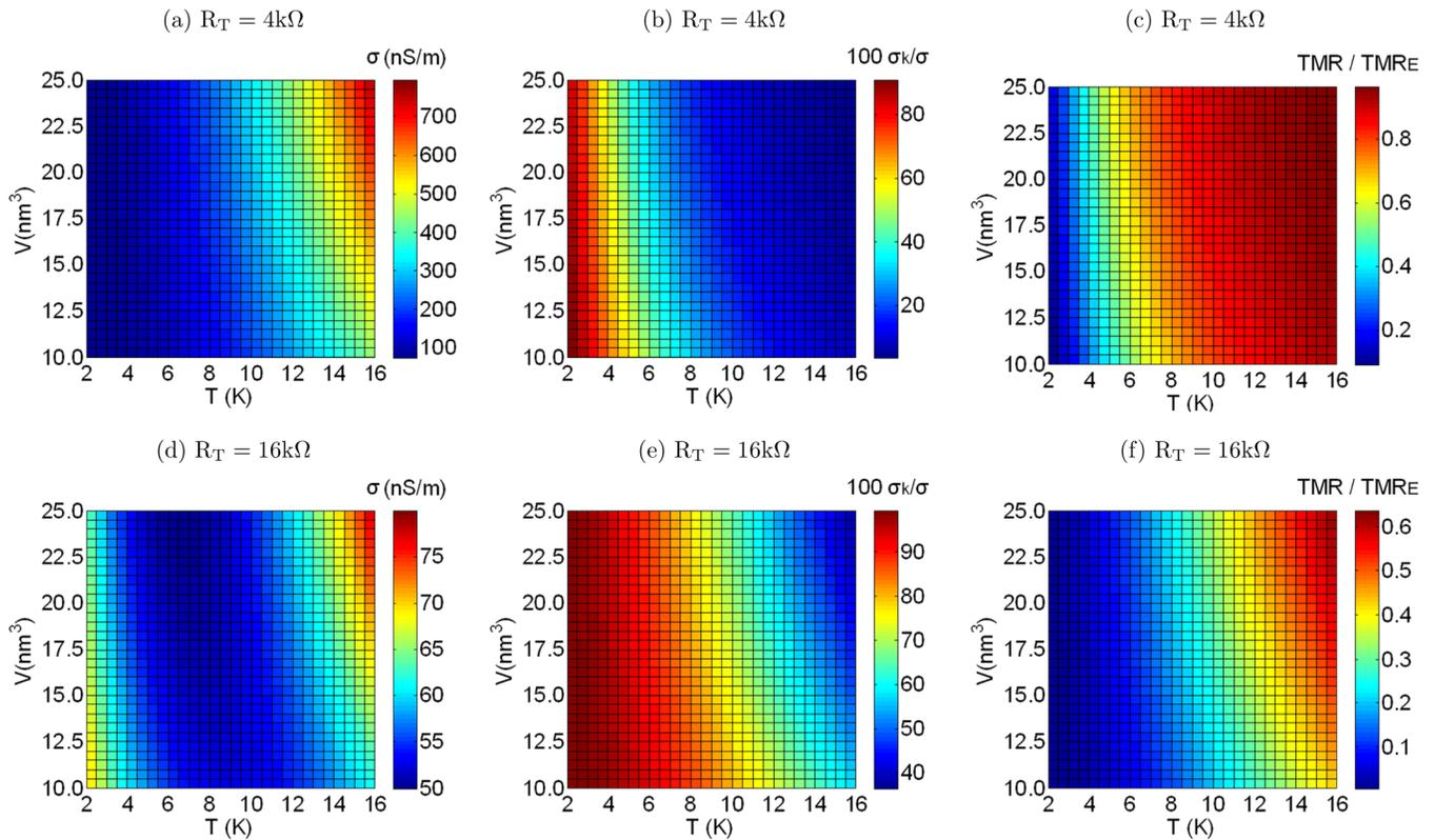
FIG. 1. Magnetotransport parameters as a function of temperature and the volume of the cluster within the barrier, for two different values of the tunnel resistance  $R_T$ . For  $R_T = 4k\Omega$  it is given the conductivity (a), the relative contribution of the Kondo conductance to the total conductance (b), and the magnetoresistance normalized by the contribution of the elastic conduction (c). The same parameters are shown in (d)–(f) for  $R_T = 16k\Omega$ .
