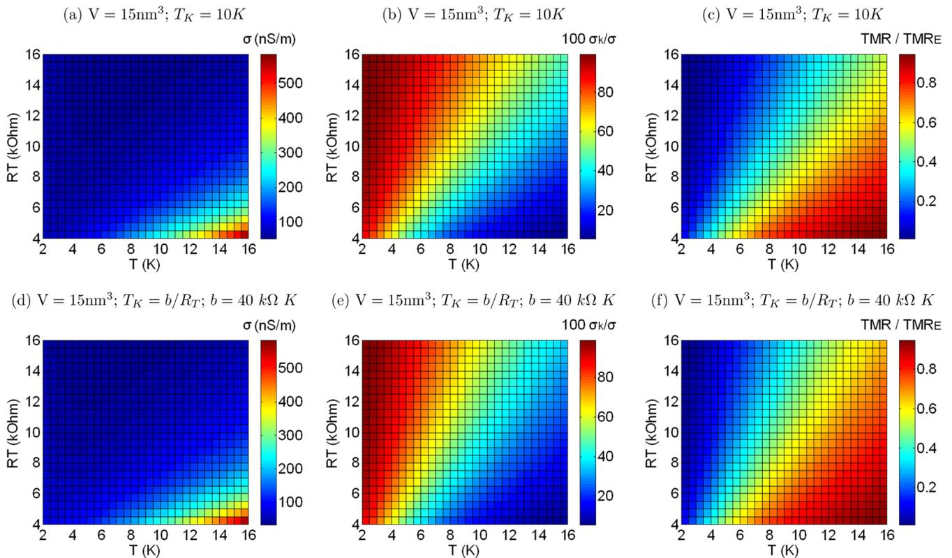
FIG. 2. Magnetotransport parameters as a function of temperature and the tunnel resistance. (a)–(c) show the conductivity, the relative contribution of the Kondo conductance to the total conductance, and the magnetoresistance normalized by the contribution of the elastic conduction, considering a constant value of the Kondo temperature  $T_K$ . The same parameters are shown in (d)–(f) supposing an exponential dependence with the barrier thickness.
