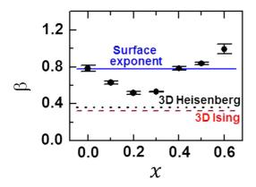
FIG. 9. (Color online) Al<sub>2</sub>O<sub>3</sub> concentration x dependence of the extracted critical exponent  $\beta$ . The straight (blue) line indicates the surface exponent predicted by Binder *et al.*, the (black) dotted line indicates the 3D Heisenberg model value, and the dashed (red) line shows the 3D Ising model  $\beta$  [31–33].
