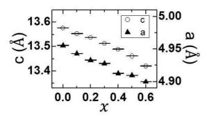
FIG. 4. Al<sub>2</sub>O<sub>3</sub> concentration x dependence of the Cr<sub>2-x</sub>Al<sub>x</sub>O<sub>3</sub> lattice parameters, determined from XRD  $\theta$ -2 $\theta$  measurements.
