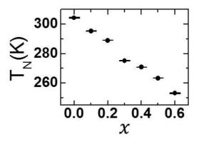
FIG. 8. Al<sub>2</sub>O<sub>3</sub> concentration x dependence of the extracted critical temperature  $T_{\rm N}$  values.
