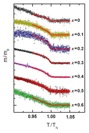
FIG. 7. (Color online) Temperature dependence of the remanent boundary magnetization in  $Cr_{2-x}Al_xO_3$  thin films of varying  $Al_2O_3$  concentration x. The (red) lines show least-squares fits to Eq. (1) for each of the sample data sets.
