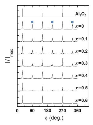
FIG. 5. (Color online) XRD  $\phi$  scans at the  $2\theta$  pole of the (10–14) planes for various  $Cr_{2-x}Al_xO_3$  thin films and for the  $Al_2O_3$  substrates. The stars mark the twinned domain positions.
