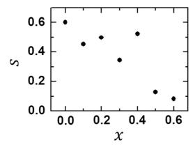
FIG. 6. Al<sub>2</sub>O<sub>3</sub> concentration x dependence of s, the ratio between the average XRD intensity of the twinned domain signal  $I_{\text{Twinned}}$  and the untwinned domain signal  $I_{\text{Untwinned}}$ , both measured for the (10–14) plane.
