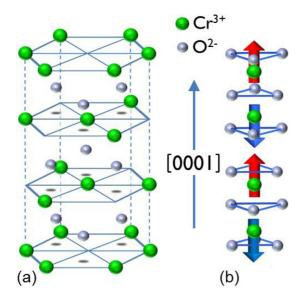
FIG. 1. (Color online) (a) Corundum crystal structure of  $\alpha$ -Cr<sub>2</sub>O<sub>3</sub>; (b) schematic of the antiferromagnetic (AFM) spin order. In zero magnetic field, the chromium spins are aligned antiparallel along the [0001] direction (c axis).
