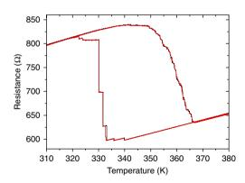
Figure 2 | Reproducibility of the resistance scans. Dependence of resistance versus temperature for a 50-nm-thick, 220-nm-wide and 2.6- $\mu$ m-long stripe. The transition upon heating is continuous and uncorrelated, whereas upon cooling the transition occurs in a few abrupt steps. Two hysteresis loops (black and red curves) measured in a sequence are plotted showing an excellent reproducibility upon temperature sweeping.
