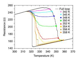
Figure 4 | Temperature-driven hysteresis loops for an FeRh stripe.
