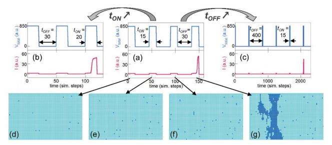
**Figure 4.** a–c) Modeling of resistive switching obtained with trains of short pulses of various  $t_{ON}$  and  $t_{OFF}$ . d–g) Snapshots of the microscopic state of the resistor network during each of the four pulses shown in panel (a). We observe that the formation of the conductive bridge is a sudden process, which occurs within the duration of a single pulse, i.e., in that case the fourth one.
