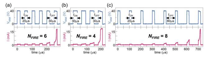
Figure 2. Experimental resistive switching obtained by applying trains of short pulses of various  $t_{ON}$  and  $t_{OFF}$ . a) Using  $t_{ON} = 20 \,\mu s$  and  $t_{OFF} = 30 \,\mu s$ leads to  $N_{\rm FIRE} = 6$ . b) Increasing  $t_{\rm ON}$  to 30  $\mu$ s leads to a decrease of  $N_{\rm FIRE}$  to 4. c) Increasing  $t_{\rm OFF}$  to 80  $\mu$ s leads to an increase of  $N_{\rm FIRE}$  to 8.
