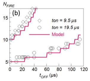
**Figure 6.** Evolution of the number of pulses necessary to a) "fire" the Mott Neuron versus the pulse duration  $t_{\rm ON}$  and b) the separation time between pulses  $t_{\rm OFF}$ . Remarkably, the parameter-free theoretical prediction established for the LIF model (see Equation (5) in the text), shown as red curves, nicely reproduces the experimental dependences.
