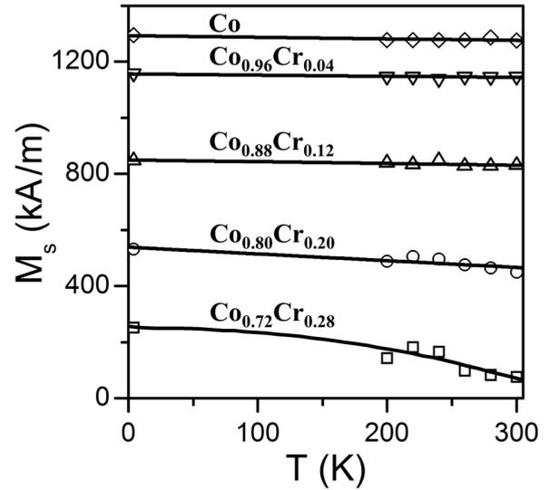
FIG. 10. Temperature dependence of the saturation magnetization for layers in the bathtub structure as determined from PNR for the sample with Cr concentration  $x_c = 0.28$ . Solid curves are guides to the eye. The open symbols include the error bars corresponding to  $\pm 1$  standard deviation.
