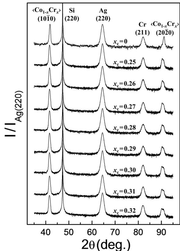
FIG. 2. XRD  $\theta$ - $2\theta$  scans for different samples with Cr concentrations  $x_c$  showing  $\langle \text{Co}_{1-x}\text{Cr}_x \rangle (10\bar{1}0)$ ,  $\text{Ag}(220)$ ,  $\text{Cr}(211)$ , and  $\langle \text{Co}_{1-x}\text{Cr}_x \rangle (20\bar{2}0)$  diffraction peaks, in addition to the  $\text{Si}(220)$  substrate signal. Each scan has been normalized to the intensity of its  $\text{Ag}(220)$  peak.
