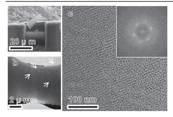
**Figure 3.** SEM and TEM images of a thin section of  $Fe_3O_4$ –ferritin crystal fabricated by FIB. (a) SEM image of a thin section of a  $Fe_3O_4$ –ferritin crystal fabricated by FIB. (b) Low magnification TEM image of the thin section from (a) on a TEM grid. White arrows show the holes of the holey carbon TEM grid. (c) High magnification TEM image of the upper central area of the thin section in (b) with FFT (inset).
