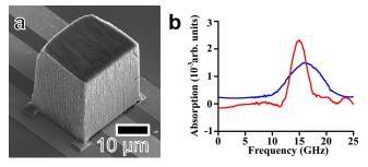
**Figure 4.** A SEM image and microwave absorption spectra of a cubic  $Fe_3O_4$ –ferritin crystal fabricated by FIB. (a) SEM image of a cube cut from an insulating  $Fe_3O_4$ –ferritin crystal fixed to the two outer ground lines of a coplanar waveguide (light-gray leads). (b) Microwave absorption spectra taken in an external magnetic field of 0.5 T applied in a direction perpendicular to the substrate (red line: 290 K, blue line: 5 K).
