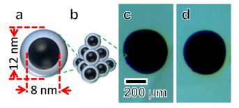
**Figure 1.** Schematic and images of  $Fe_3O_4$ –ferritin crystals. (a) Schematic of monomer of  $Fe_3O_4$ –ferritin. (b) Schematic of crystals of  $Fe_3O_4$ –ferritin and optical images of crystals of  $Fe_3O_4$ –ferritin before (c) and after chemical fixation (d). Green broken lines show the scale relationship between the schematics and the image.
