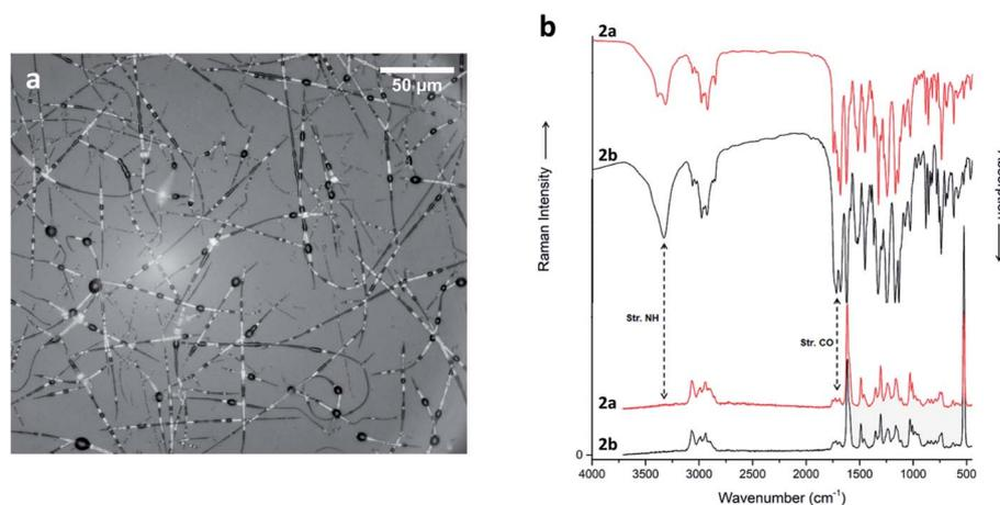
Fig. 6 (a) Optical micrographs of compound **2a** electrospun nanofibers ( $15\text{ cm}$ ,  $15\text{ kV}$ ,  $0.5\text{ ml h}^{-1}$ ), recorded in air in reflection (the strong contrast in the fibers results from various distances from the Si wafer substrate). (b) Raman (bottom) and IR spectra (top) of compounds **2a** (black) and **2b** (red) powder. Spectra are scaled and offset for clarity.
