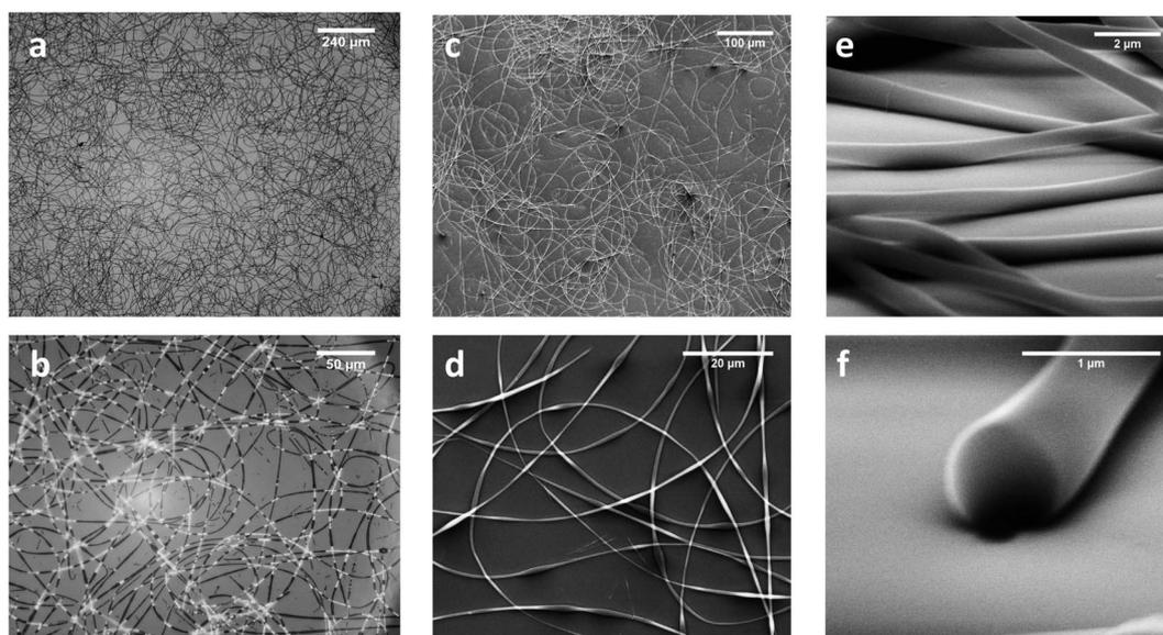
Fig. 3 (a and b) Optical micrographs of compound **1** electrospun nanofibers ( $15\text{ cm}$ ,  $15\text{ kV}$ ,  $0.5\text{ ml h}^{-1}$ ); (c and d) SEM micrographs of compound **1** nanofibers; (e) also observed under tilt of  $75^\circ$ ; (f) cross section of the fiber. SEM was recorded in vacuum (voltage 2–10 kV), optical images in air.
