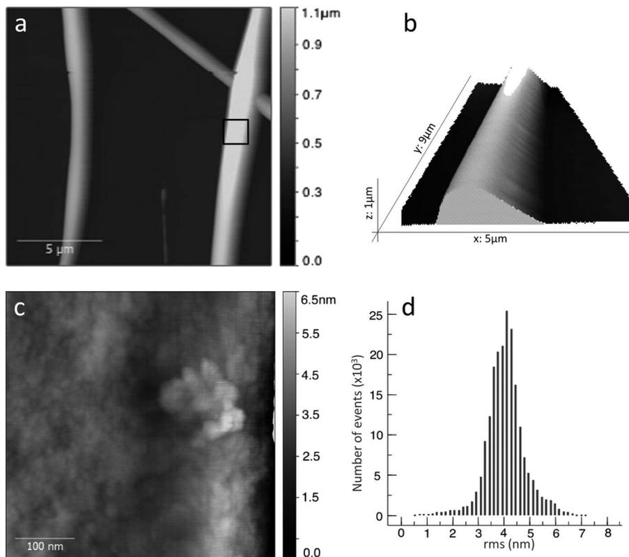
Fig. 4 AC mode (tapping) AFM scans of compound 1 electrospun nanofibers (15 cm, 15 kV, 0.5 ml h<sup>-1</sup>). (a) topography image of compound 1 nanofibers on a silicon wafer substrate, overview; (b) 3D rendering of a fiber detail; (c) zoom into area indicated in (a); (d) height distribution for (c).
