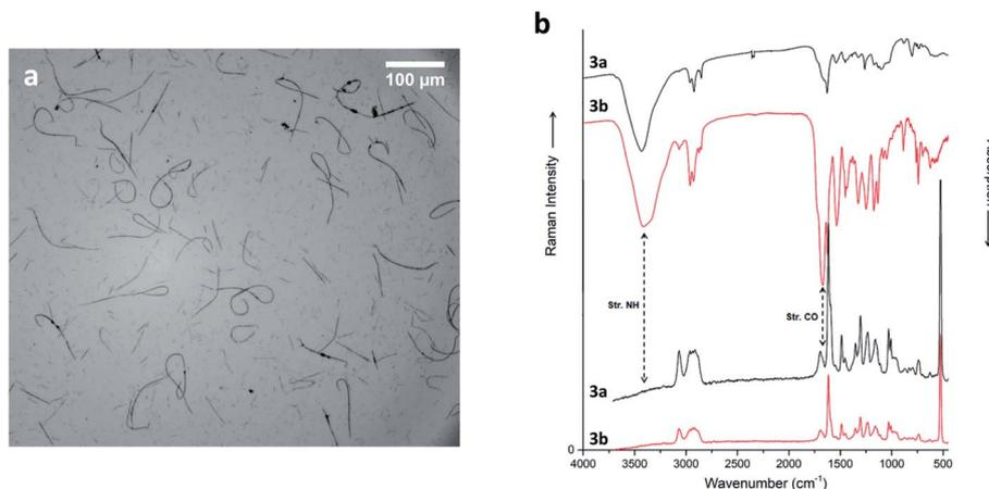
Fig. 7 (a) Optical micrograph of compound **3b** electrospun nanofibers (15 cm, 15 kV, 0.5 ml h<sup>-1</sup>), recorded in air. (b) Raman (bottom) and IR spectra (top) of compounds **3a** (black) and **3b** (red) powder. Spectra are scaled and offset for clarity.
