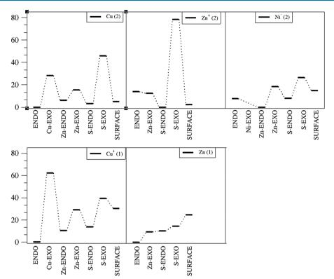
Figure 7. Energy profiles of all the TM doped  $(ZnS)_{12}$ , in which the TMs have either  $4s^{1}d^{10}$  (top) or  $4s^{2}d^{10}$  (bottom) electronic structure.
