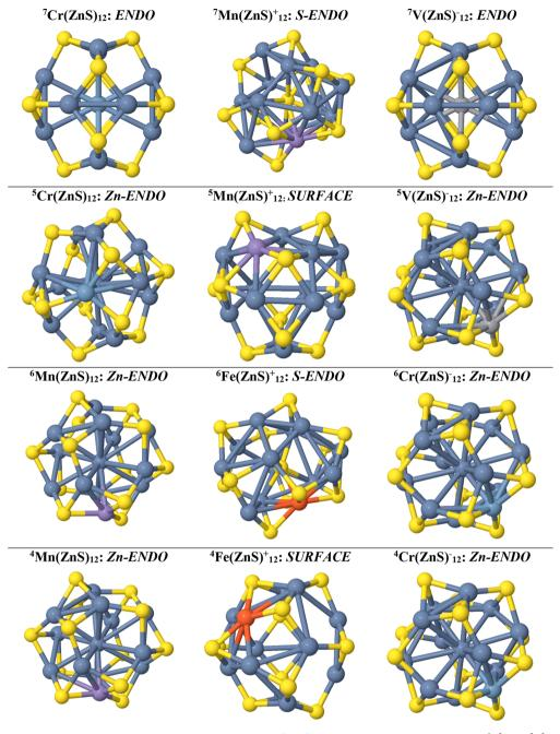
Figure 6. Most stable high- and low-spin structures for all the TM doped  $(ZnS)_{12}$ , in which the TMs have either  $4s^1d^5$  or  $4s^2d^5$  electronic structure.
