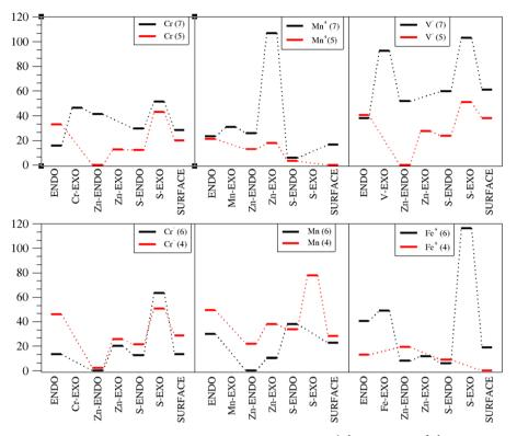
Figure 5. Energy profiles of all the TM doped  $(ZnS)_{12}$ , in which the TM has either  $4s^1d^5$  (above) or  $4s^2d^5$  (below) electronic structure.
