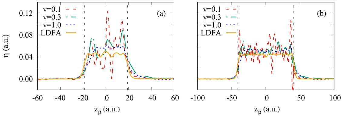
Fig. 4 Friction coefficient for the antiproton crossing (a)  $\text{Na}_{106}$  and (b)  $\text{Na}_{1074}$  cluster. Different curves correspond to the results obtained for different antiproton velocities  $v$  as indicated in the insert, where  $v$  is given in atomic units. The orange curve denoted as "LDFA" shows the friction coefficient calculated within the LDFA approximation. Vertical dashed lines indicate the border of the positive background of the jellium cluster.
