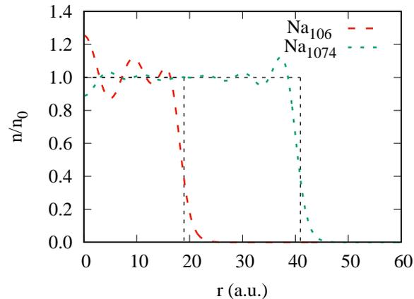
Fig. 9 Ground state electron density profile of the spherical clusters  $\text{Na}_{106}$  and  $\text{Na}_{1074}$  in the units of the constant background density  $n_0$  (thin dashed line) as a function of the radial coordinate.
