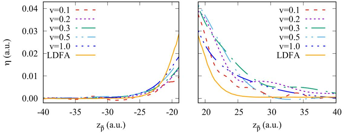
Fig. 7 Friction coefficient for the antiproton moving in vacuum outside the  $\text{Na}_{106}$  cluster. The in-going (left panel) and out-going (right panel) trajectory segments are shown. Different curves correspond to the results obtained for different antiproton velocities  $v$  as indicated in the insert, where  $v$  is given in atomic units. The orange curve denoted as "LDFA" shows the friction coefficient calculated within the LDFA approximation.
