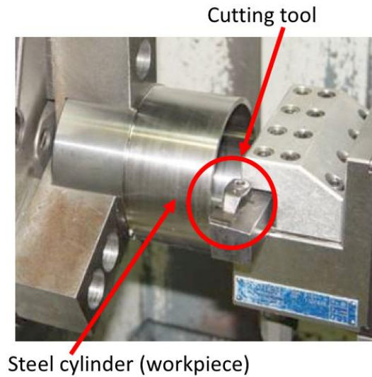
Figure 3-27 Setup for steel machining by turning a workpiece in form of cylinder.
