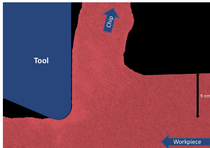
Figure 7-3 Workpiece cut and chip generation in case of 9 nm of feed. The tool of use has 4 nm of radius.
