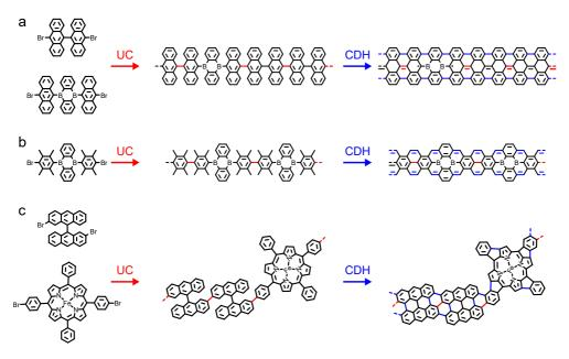
Figure 1.2: Molecular precursors and envisioned synthesis route for the investigated nanoribbons: a, b, c Lewis structures of (left to right) the molecular precursors, the Ullmann-coupled polymer and the planar GNR corresponding to the ribbon used in Chapter 2–4 (a), Chapter 5 (b) and Chapter 6 (c). Submonolayers of the molecular precursors were codeposited on the sample held at room temperature before the thermal activation of the reaction steps.
