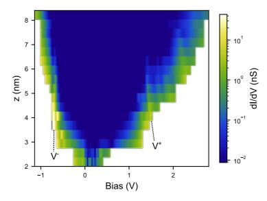
Figure 2.10: Conductance map of the pristine 7aGNR Colorplot of  ${\rm d}I/{\rm d}V$  spectra at different tip sample separation z in logarithmic scale.
