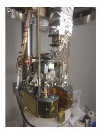
**Figure 1.3:** Laboratory and Slider Head: a,b Picture of the UHV low-temperature scanning tunneling microscope system and CreaTec slider head used in this Thesis.
