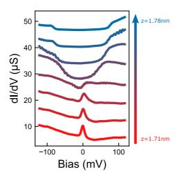
Figure 5.5: Transition from Kondo to IET regime: A Stack of differential conductance spectra taken in steps of  $\Delta z=10\,\mathrm{pm}$  shows the continuous transition from the Kondo resonance to a IET excitation. Data corresponding to Figure 5.4e. The spectra are offset by  $6.6\,\mu\mathrm{S}$  for clarity.
