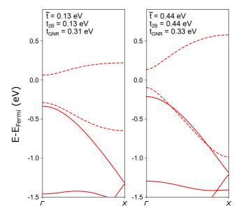
Figure 4.8: MFH band structures used for fitting the SSH model: Band structure of the periodic 2B-7aGNR obtained by MFH calculations with a hybridization of  $\tilde{t}=0.13\,\mathrm{eV}$  (left) and  $\tilde{t}=0.44\,\mathrm{eV}$  (right). The frontier bands are indicated by the dashed lines. The SSH parameters extracted from the band structure are given in the plot.
