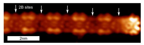
Figure 4.5: Edge state in a (2B)<sub>d</sub>-GNR: STM constant height current image of the edge state of a densely 2B-doped GNR. ( $V_{\rm b}=5\,{\rm mV}$ ).
