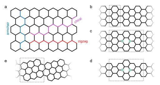
**Figure 1.5: Graphene and graphene nanoribbons: a** Graphene is formed by  $sp^2$  hybridized carbon atoms that form a honeycomb lattice. Graphene nanoribbons, one dimensional narrow stripes of graphene are classified by their edge structure as armchair, zigzag or graphene nanoribbons. **b–e** Atomic structure of the different GNRs investigated in this Thesis and their respective unit cell (dashed, grey rectangle). **b** 7aGNR, **c** 2B-7aGNR, **d** 2B-575-aGNR, **e** (3,1)-chiral GNR.
