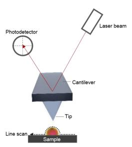
**Figure 2.11. Atomic Force Microscopy (AFM) basic components.** The tip and the sample surface constitute the sensor and the detection system is formed by the photodetector and the laser beam. Note that the tip movement across the sample is controlled by a piezoelectric material.
