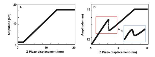
**Figure 2.15.** Amplitude versus z-piezo displacement curves typically obtained by AFM. (A) The amplitude is controlled by long-range attractive forces. (B) The amplitude exhibits a local maximum due to the competition of long-range attractive and short-range repulsive forces. Note that the local maximum can be step-like (red square) or smooth (blue square)
