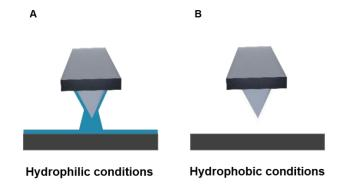
Figure 2.14. AFM measurements in intermittent contact mode (AC mode) under different conditions. (A) AFM performed with a hydrophilic tip and a hydrophilic sample, where a capillary neck is formed. (B) AFM performed with a hydrophobic tip and a hydrophobic sample, where no capillary neck is formed.
