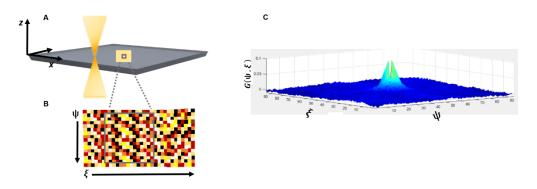
Figure 2.10. Principle of RICS. (A) A single frame is taken in 2-dimensions. (B) Pixel scans can be arranged in 2-dimensions to form a pseudo-image. (C) Experimental correlation curve  $G(\psi, \xi)$  obtained from the pseudo image and fitted to a 2-dimensional flow-diffusion model.
