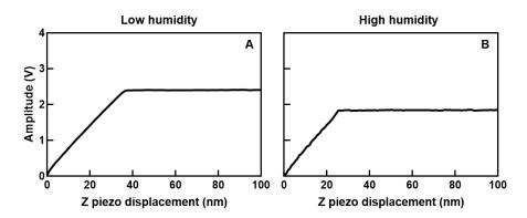
**Figure 3.9. Cantilever oscillation amplitude versus z-piezo displacement on hydrophilic conditions obtained by AFM.** (A) Representative curve obtained at low humidity (~ 15 % relative humidity, RH). (B) Representative curve obtained at high humidity (~ 95 % RH). Note that in both cases the free amplitude (A<sub>0</sub>) was 4 V, which corresponds to the maximum value in the display chart.
