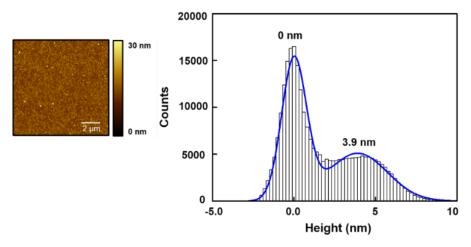
Figure 4.12. AFM topography image and height histogram of HA-bilayers after dehydration. The height histogram was fitted to a 2-peak Gaussian function (number of images, n = 16). The estimated height difference from the main peaks was considered as the depth of the lipid bilayer in the dehydrated state. Note that the height data provided by the AFM are not absolute values. Hence, we assigned arbitrarily the average height of the substrate underneath the bilayer to the value zero.
