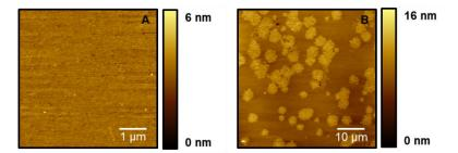
**Figure 2.12. AFM topography image of a SLB in solution**. (A) SLB deposited on mica where slight nanometric variations in signal are detected and converted into a color mapping. (B) SLB after the addition of HA where variations in signal intensity are evident. Note that differences in intensity colors suggest in (A) a homogenous and flat SLB on mica (light brown image) and in (B) a flat mica surface (dark brown) with HA bound to SLB patches (light brown structures).
