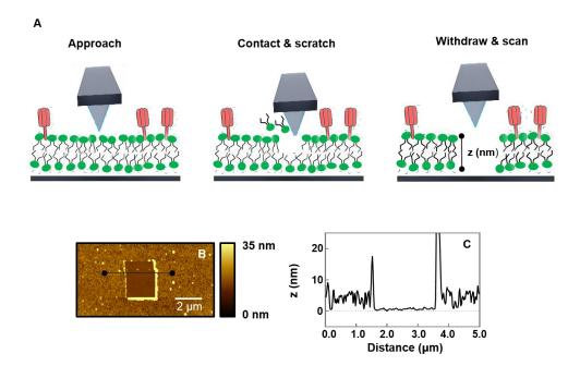
**Figure 4.13. AFM scratch and scan test performed on HA-bilayers**. (A) Representative scheme of the scratch and scan test: The tip approaches the sample surface till contact occurs. Scratching is performed in AFM contact mode at high setpoint values. Lately, the tip is withdrawn and the sample is scanned in tapping mode. (B) AFM topography image of a scratched region on DOPC 90 mol % and DGS-NTA-Ni 10 mol % SLB containing HA. (C) Height profile extracted from the horizontal line in (A).
