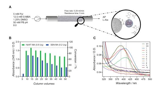
Figure 7-10. Continuous flow deamination by immobilized HeWT/HeWT@pAA-NH<sub>2</sub> on epoxy-methacrylate supports. (A) Schematic of the flow system setup with immobilized HeWT@pAA-NH<sub>2</sub> loaded with PLP. (B) The operational performance of the packed bed reactors. (C) UV-Vis spectra of the 2 washings (W) and first 10 column volumes of HeWT@pAA-NH<sub>2</sub> sample.
