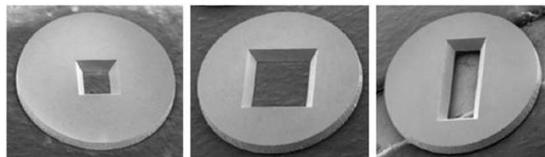
Figure 3.13. SEM images of Si discs (3mm in diameter) with  $\text{Si}_3\text{N}_4$  membranes of different sizes. The images show a view of the windows etched into the Si substrate at the back side of the membranes. (taken from www.Ted Pella.com).
