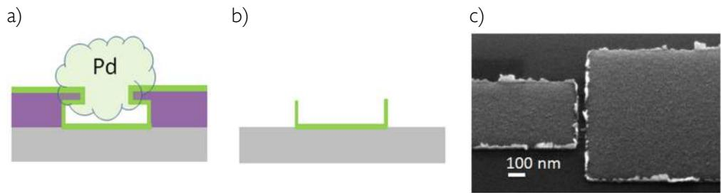
Figure 2.7. Formation of metallic fringes by sputtering. a) Sketch representing the deposition of palladium by sputtering. b) Metal deposited on the resist walls leads to fringes remaining after lift off. c) Example of closely spaced electrodes with a shortcut occasioned by the remaining metallic fringes.
