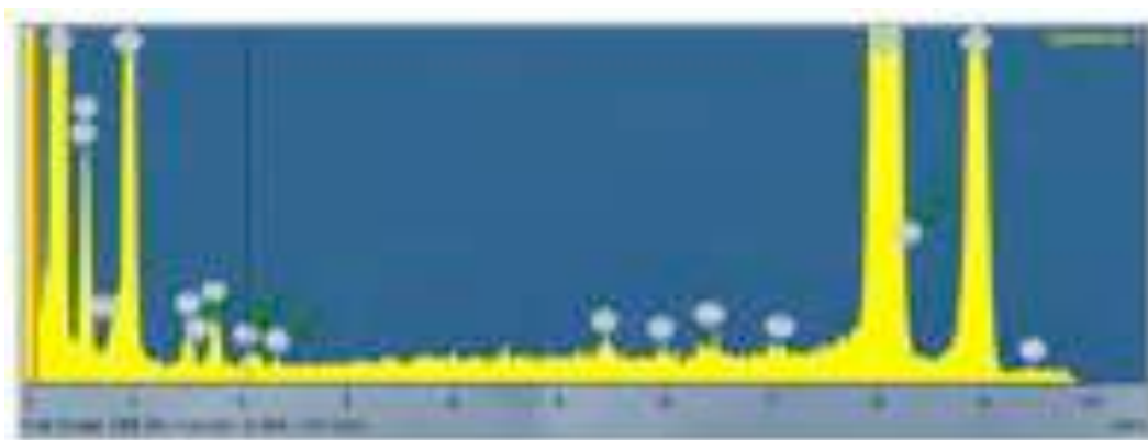
Figure 5.4.5. EDX spectra of oxaliplatin encapsulated TMV particles. Pt peaks are shown with green arrows. No Cl peaks were seen unlike cisplatin since oxaliplatin does not have Cl ligands. Cu and C peaks are coming from the TEM grids. Fe, Cr, Si and Al peaks originate from the sample holder of the microscope.
