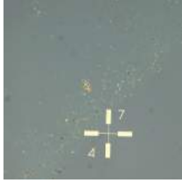
Figure 6.2: Optical picture of the residues on the SiO 2 /Si substrate after the exfoliation and transfer of MoS 2 with scotch tape.
