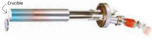
Figure 3.10: Picture of a cold-lip effusion cell, used in this thesis for thermal evaporation. The location of the crucible inside the cell is indicated. Figure taken from Ref. 238.
