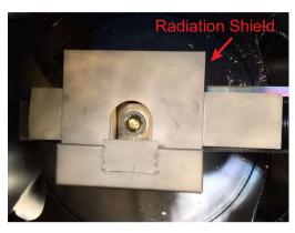
**Figure 2.4** | **Inner view of the metal chamber. a**, Photo of the e-beam evaporator of the metal chamber. The filament emits electrons, which are accelerated by a high voltage and deflected by permanent magnets towards the evaporation material. **b**, Picture of the radiation shield.
