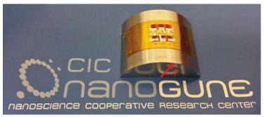
**Figure 5.1** | **A sample holder.** The photography shows a bent flexible chip on Kapton with six i-MOS devices. The sample is pasted on a half cylinder that works as sample holder and that permits performing measurements under applied strain.
