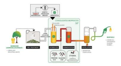
Figure 1.10. Enzymatic lignocellulose conversion process into valuable products such as bioethanol.
