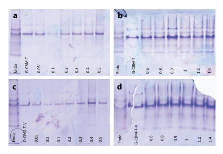
Figure 5.28. Native gel of the complex form between Endo-DockT and the cellulosome scaffold. The number below represents the scaffold/enzyme ratio used in each case.
