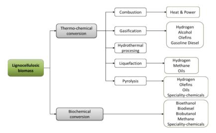
Figure 1.9. Thermochemical and biochemical processing of lignocellulosic biomass [68].
