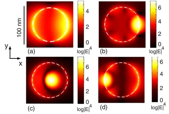
FIG. 7. (Color online) Fourth power of the calculated local field enhancement normalized to the incoming field on top of a gold nanodisk for four different positions of a strongly interacting dipolar probe: (a) far edge at 41 nm on top of the disk, (b) far edge at 21 nm on top of the disk, (c) center at 21 nm on top of the disk, and (d) near edge at 21 nm on top of the disk.
