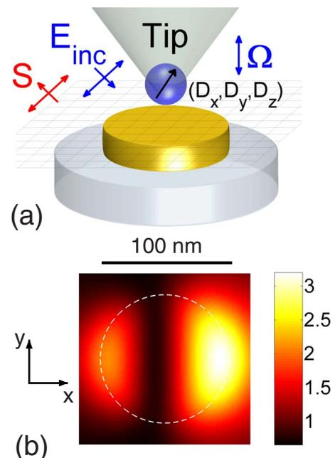
FIG. 1. (Color online) (a) Schematics of the near-field imaging process. A tip located at position  $(D_x, D_y, D_z)$  scans the nanoantenna under study (gold nanodisk). We define  $D_x=0$ ,  $D_y=0$ , and  $D_z=0$  to be at the center of the disk on the top surface. Incident light  $E_{inc}$  illuminates the tip-antenna system and backscattered far-field amplitude  $s$  is recorded. (b) Calculated near-field amplitude on top of a gold nanodisk in absence of the tip.
