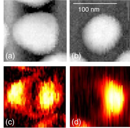
FIG. 3. (Color online) [(a) and (c)] Topography and near-field amplitude signal  $s_3$  of a gold nanodisk obtained with use of a CNT tip. [(b) and (d)] Topography and near-field amplitude signal  $s_3$  obtained with use of a Pt-coated Si tip.
