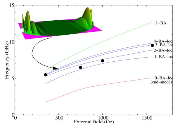
FIG. 1. (Color online) Frequencies of selected spin modes calculated as a function of the applied field with a cell size 10 nm (lines), plotted together with the experimental points of the commented letter (dots). The inset shows the magnetization profile ( $|m_z|$ ) of the 3-BA-loc mode at 500 Oe.
