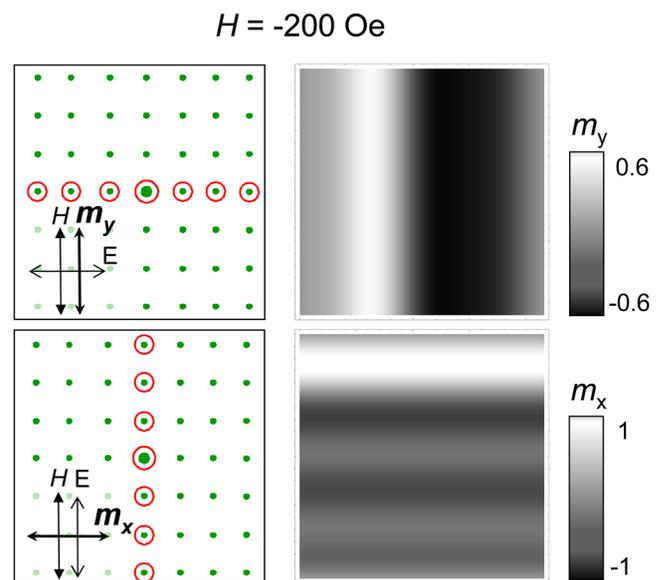
FIG. 3. (Color online) Spatial map of the magnetization profile in the unit cell of the array at  $H = -200$  Oe reconstructed via inverse Fourier transform using the form factors of Fig. 2. The left column shows a schematic of the diffraction pattern with the beams used for the reconstruction (marked by circles).
