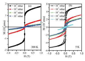
FIG. 1. (Color online) Magnetic moment as a function of applied field at room temperature (a) and at  $5~\mathrm{K}$  (b) for the films prepared at different partial pressures.
