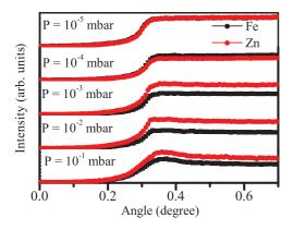
FIG. 2. (Color online) Intensity of Fe and Zn  $K\alpha$  lines as a function of incident angle for all films. The intensities are in arbitrary units.
