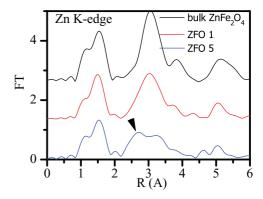
FIG. 6. (Color online) Fourier transforms of  $k^2\chi(k)$  oscillations (Zn K edge) of bulk ZnFe<sub>2</sub>O<sub>4</sub>, ZFO1, and ZFO5 film ferrites. The arrow indicates the new coordination appearing in the FT of sample ZFO5, which indicates that there are Zn atoms at B sites.
