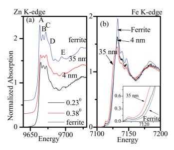
FIG. 4. (Color online) (a) Zn and (b) Fe K edge XANES, taken for film deposited at  $10^{-4}$  mbar for two different incidence angles.
