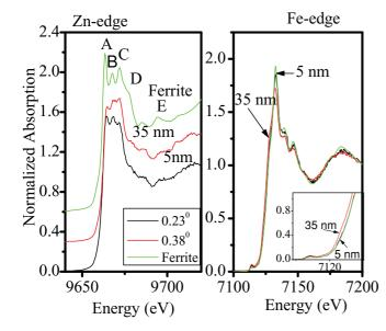
FIG. 5. (Color online) (a) Zn and (b) Fe K-edge XANES, taken for film deposited at  $10^{-1}$  mbar for two different incidence angles.
