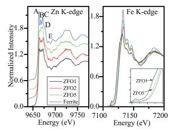
FIG. 3. (Color online) (a) Zn and (b) Fe K-edge XANES using an incident angle of  $0.38^{\circ}$  for films deposited at different oxygen pressures.
