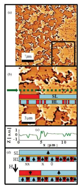
FIG. 5. (Color online) (a) MFM image of the remanent domain structure during down reversal. (b) Zoom into previous image. Inset: Sketch of the domain structure in soft layer (SL) and hard layer (HL) along an arbitrarily chosen green line of the MFM scan reconstructed from (c) the contrast Z of the image along same line. (d) Sketch of the reversal process.
