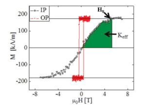
FIG. 3. (Color online) SQUID magnetometry in-plane (IP) and out-of-plane (OP) hysteresis loop for a  $\text{Co}_{74}\text{Tb}_{26}$  (20 nm) film. The effective anisotropy constant  $K_{\text{eff}} = K_{\text{u}} - 1/2~\mu_0~M_{\text{S}}^2$  can be approximated as the surface under the IP loop between the origin and the saturation field  $H_{\text{S}}$ .
