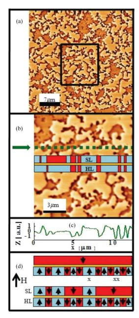
FIG. 6. (Color online) (a) MFM image of the remanent domain structure during up reversal. (b) Zoom into previous image. Inset: Sketch of the domain structure in soft layer (SL) and hard layer (HL) along an arbitrarily chosen line of the MFM scan reconstructed from (c) the contrast Z of the image along same line. (d) Sketch of the reversal process.
