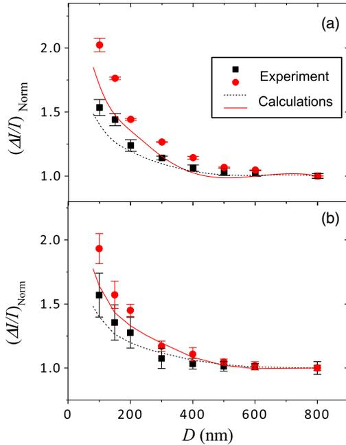
FIG. 3 (color online). Normalized transverse magneto-optical signal  $\Delta I/I$  in saturation vs disk diameter  $D$  for light of wavelength (a)  $\lambda = 532$  nm and (b)  $\lambda = 633$  nm. The experimental data for 15 nm and 25 nm thick disks are shown as (black) squares and (red) dots, respectively. The lines represent results derived from E-DDA calculations using the exact same geometry as the experiment. All data are normalized to their respective values at  $D = 800$  nm.
