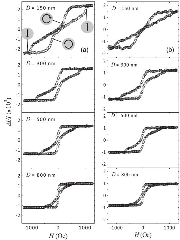
FIG. 2. Transverse magneto-optical signal  $\Delta I/I$  vs applied magnetic field strength  $H$  for samples of different diameter  $D$ , measured for light of wavelength (a)  $\lambda = 532$  nm and (b)  $\lambda = 633$  nm. The insets in the topmost figure of (a) are schematic representations of the magnetization states at different field values following a complete hysteresis loop cycle. The measurements shown here were acquired for  $m = 1$  and a sample with  $t = 25$  nm.
