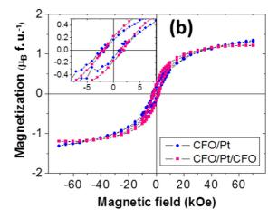
FIG. 1. (a) X-ray diffraction  $\theta$ -2 $\theta$  pattern of the STO//CFO(28 nm)/Pt/CFO(28 nm) sample. (b) Room-temperature magnetization loops for the STO//CFO(28 nm)/Pt/CFO(28 nm)/Pt samples. Inset in (b) is a zoom of the low-field region of the magnetization loops (magnetization units are Bohr magnetons per formula unit).
