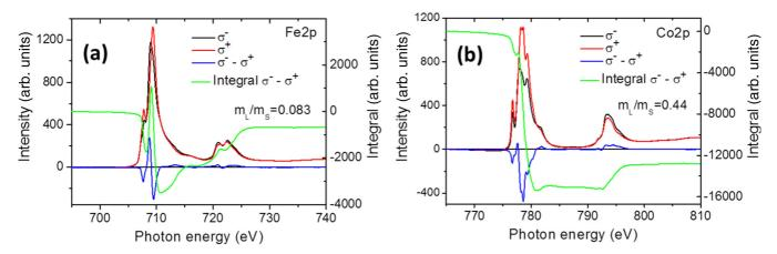
FIG. 3. (a) Fe- $L_{2,3}$  and (b) Co- $L_{2,3}$  2p XMCD spectra STO//CFO(28 nm)/Pt/CFO(28 nm) sample (295 K, 60 kOe, normal incidence). The black, red, and blue lines (left axis) show the absorption for  $\sigma^-$  and  $\sigma^+$  photon helicities and the dichroic ( $\sigma^- - \sigma^+$ ) spectra, respectively. The green line shows the integrated difference spectrum (right axis).
