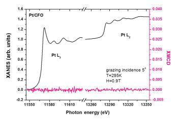
FIG. 5. X-ray absorption spectra (black line, left axis) measured across the Pt- $L_{3,2}$  atomic absorption edges of the STO//CFO(28 nm)/Pt sample. Right axis: XMCD signal.
