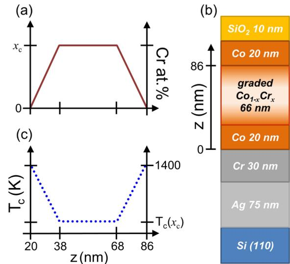
FIG. 1. (a) shows the Cr content depth profile, (b) the schematic of the layer growth sequence for the sample type studied in this work, and (c) the associated effective Curie temperature  $T_C$  depth profile for the 66-nm-thick graded  $\text{Co}_{1-x}\text{Cr}_x$  layer.  $T = 1400$  K corresponds to the  $T_C$  of pure cobalt.
