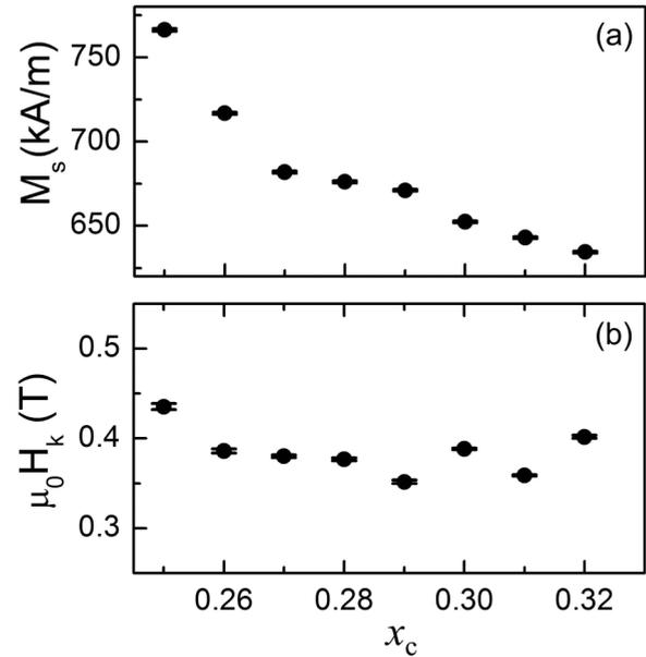
FIG. 5. Room temperature magnetic properties for the graded epitaxial Co/Co $_{1-x}$ Cr $_x$ /Co (10 $\bar{1}$ 0) samples as a function of Cr content  $x_c$ : (a) saturation magnetization  $M_S$  and (b) magnetocrystalline anisotropy field  $H_K$ .
