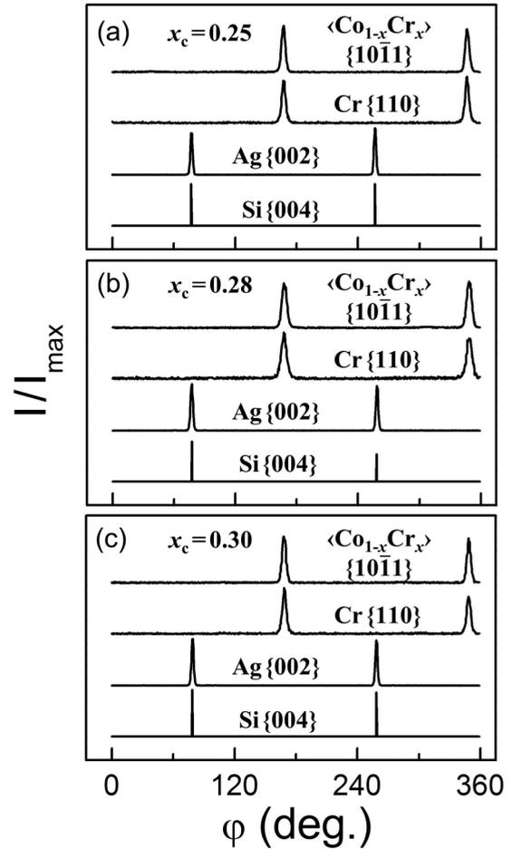
FIG. 3. XRD  $\varphi$  scans at the  $2\theta$  poles of the Si {004}, Ag {002}, Cr {110}, and  $\langle\text{Co}_{1-x}\text{Cr}_x\rangle$  {10 $\bar{1}$ 1} planes for Cr concentrations  $x_c = 0.25, 0.28, 0.30$ .
