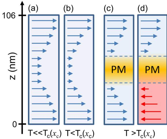
FIG. 8. Schematics of the magnetization depth profile at remanence for temperatures below (a,b) and above (c,d) the minimum effective  $T_C$ . For high temperatures, the paramagnetic (PM) region interrupts the exchange coupling through the thickness, allowing the system to be in either a parallel (c) or antiparallel (d) configuration.
