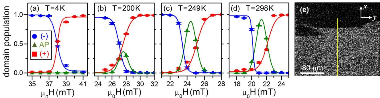
FIG. 13. (a-d) Field-dependent domain populations as determined from incoherent scattering model of the PNR data. Error bars correspond to  $\pm 2$  standard deviations. (e) Room temperature MOKE microscopy image taken during the reversal along the easy axis. Solid yellow line represents the average projection of the neutron coherence length for the PNR measurements.
