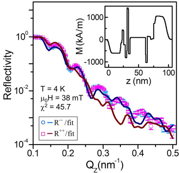
FIG. 11. PNR data measured at  $T = 4$  K in  $\mu_0 H = 38$  mT following prior saturation in a  $\mu_0 H = -700$  mT for the sample with Cr concentration  $x_c = 0.28$ . Solid lines are best fits corresponding to a model assuming coherent scattering from a single magnetic depth profile (shown inset). Error bars correspond to  $\pm 1$  standard deviation.
