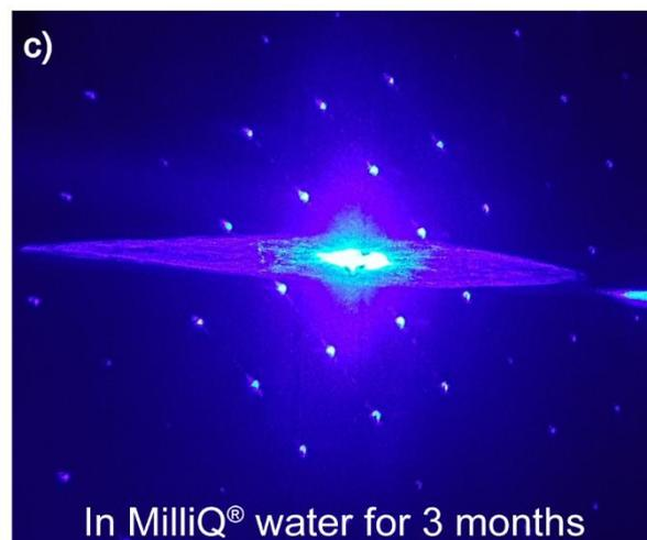
**Figure 2 – Biodegradability.** (a) Biodegradability in soil of cellulose and cocoa pod husk materials. (b) BOD data in seawater of cellulose and cocoa pod husk materials. (c) Diffraction pattern of the hexagonal cellulose PC taken with the sample in ultrapure MilliQ® water for three months.
