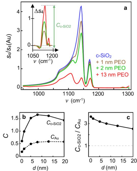
**Figure 4.8. Simulation of thickness-dependent spectra and spectral contrasts.** (a) Calculated nano-FTIR amplitude spectra of differently thick PEO layers on a quartz substrate. Inset: Spectral contrast  $\Delta S_4$  of the differently thick PEO layers, analogous to Figure 4.5. (b) Maximum spectral contrast for differently thick PEO layers on quartz and Au substrates,  $C_{\text{c-SiO}_2}$  and  $C_{\text{Au}}$  (c) Ratio  $C_{\text{c-SiO}_2}/C_{\text{Au}}$ .
