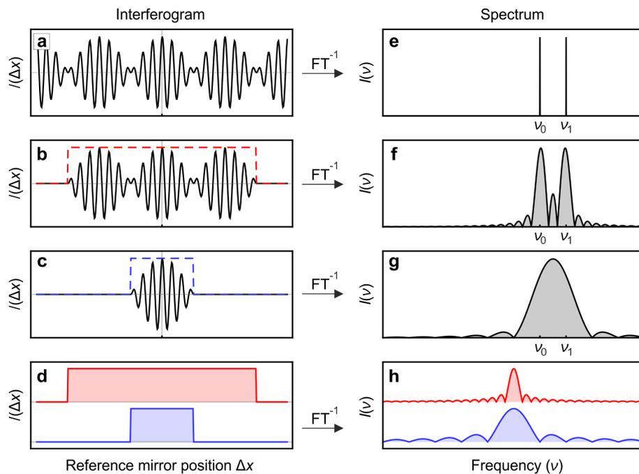
**Figure 3.15: Spectral resolution as a function of interferogram length.** (a-c) Interferograms of different length and (e-g) corresponding spectra obtained by inverse Fourier transformation ( $FT^{-1}$ ). In all cases, the same bi-chromatic light source emitting at frequencies  $\nu_0$  and  $\nu_1$  is assumed. (d) Boxcar functions that describe the finite interferogram lengths that are used in panels b and c and (h) the corresponding spectra.
