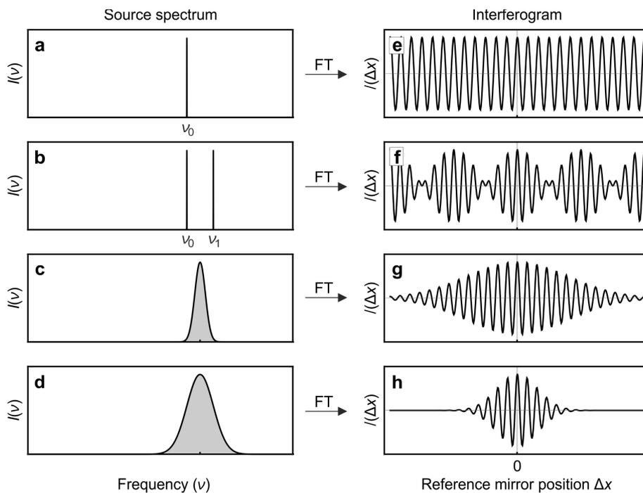
**Figure 3.14: Relation between light source spectra and corresponding interferograms.** (a-d) Light source emission spectra  $I(\nu)$  and (e-h) corresponding interferograms  $I(\Delta x)$  obtained by Fourier transformation (FT), for light sources emitting (a,e) at frequency  $\nu_0$ , (b,f) at frequencies  $\nu_0$  and  $\nu_1$ , (c,g) a spectrally narrow Gaussian intensity distribution and (d,h) a spectrally broad Gaussian intensity distribution.
