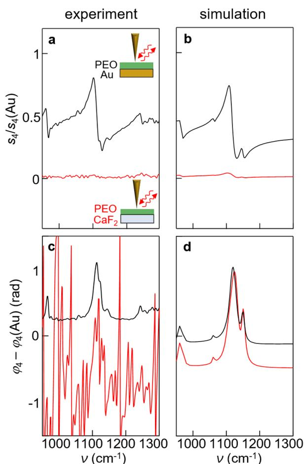
**Figure 4.2. nano-FTIR spectroscopy of 13 nm thick PEO layers on  $\text{CaF}_2$  and Au substrates.** (a,c) Experimental amplitude (a) and phase (c) spectra of 13 nm-thick PEO on Au (black curve) and  $\text{CaF}_2$  substrate (red curve). (b,d) Calculated spectra, analogous to panels a,c. All spectra are normalized to the nano-FTIR spectrum of a bare Au sample.
