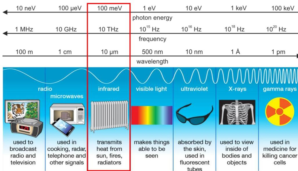
**Figure 3.1: Electromagnetic spectrum.** Different types of electromagnetic radiation are characterized by their photon energy, frequency and wavelength and are sensitive to various material properties (as illustrated). Importantly, the infrared spectral range is also highly sensitive to molecular vibrations which allows for chemical identification of materials. Figure adapted from [33].
