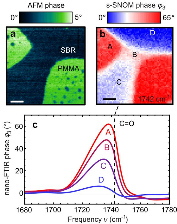
**Figure 5.3: Near-field imaging and spectroscopy of organic nanocomposites.** (a) AFM mechanical phase image of a two-component rubber blend (SBR/PMMA) and (b) corresponding s-SNOM phase  $\varphi_3$  image recorded at  $1742\text{ cm}^{-1}$ , which maps the absorption of the C=O vibrational mode of PMMA. Scale bar: 200 nm. (c) Nano-FTIR phase  $\varphi_3$  spectra of selected positions A - D. Vertical dashed line marks the imaging frequency.
