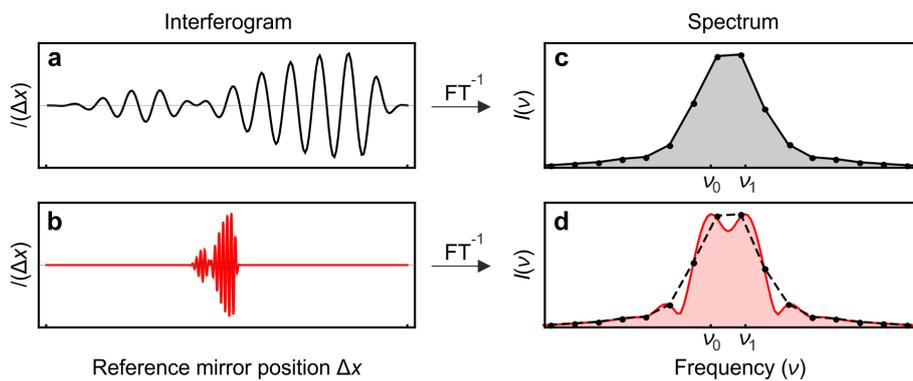
**Figure 3.17: Zero-filling of the interferogram increases the apparent spectral resolution.** (a) Interferogram without zero-filling and (b) with zero-filling using a fill-factor of 7. (c-d) Corresponding spectra obtained by inverse Fourier transformation ( $FT^{-1}$ ). The dashed line in panel d shows the same data points as panel c.
