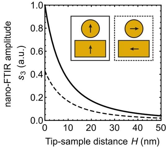
**Figure 3.7: Approach curve calculated by PDM.** Nano-FTIR amplitude  $s_3$  as a function of tip-sample distance  $H$ , calculated for a vertically oriented dipole (solid curve) and a horizontally oriented dipole (dashed curve). Calculated for a gold tip and gold sample with permittivity  $\epsilon_s = -5000+i1000$ , tip radius  $R = 30$  nm, tip tapping amplitude  $A = 30$  nm and demodulation order  $n = 3$ .
