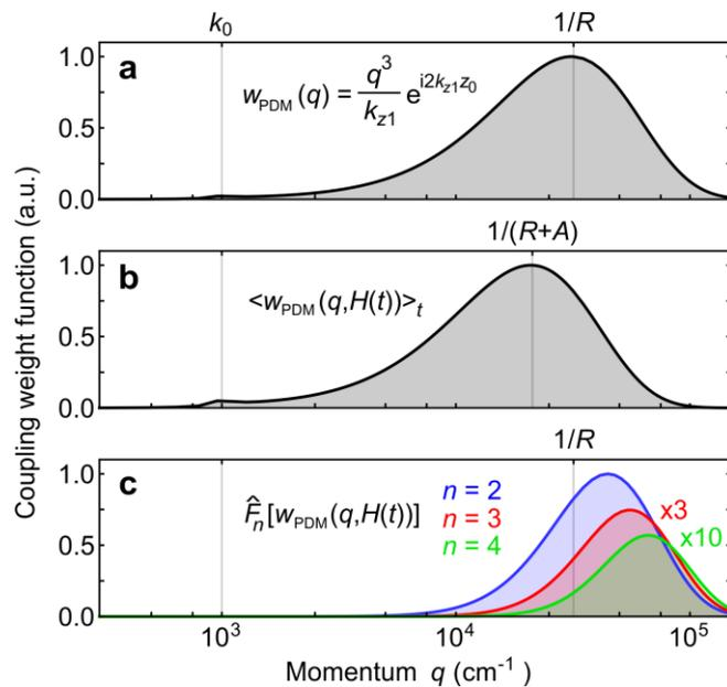
**Figure 3.12: Variations of the coupling weight function (CWF).** CWF of the PDM for layered samples. (a) Plotted for  $H = 1$  nm. (b) Time-averaged CWF  $\langle w_{\text{PDM}}(q, H(t)) \rangle_t$  over one oscillation cycle of the tip modulation  $H(t)$  with tapping amplitude  $A = 25$  nm. (c) Demodulated CWF for  $A = 25$  nm and demodulation orders  $n = \{2, 3, 4\}$ . (a-c) Tip radius  $R = 50$  nm.
