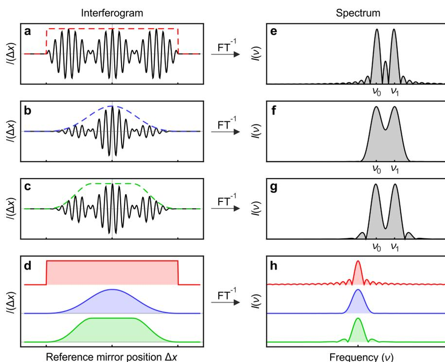
**Figure 3.16: Varying apodizations of the same interferogram.** (a-c) The same interferogram is multiplied by various apodization functions (dashed lines) and (e-g) corresponding spectra obtained by inverse Fourier transformation ( $FT^{-1}$ ). (d) Apodization functions used in panels a-c and (h) their corresponding spectra.
