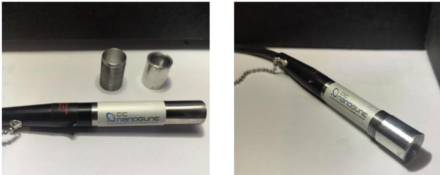
Figure 5.6: Implementation of an opto-mechanical module to the RamanProbe™ that allows for contact measurements.
