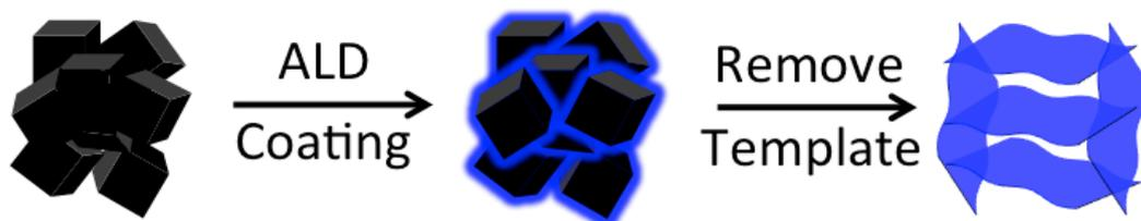
Figure 3.8 Schematic of synthesizing nanosheets by ALD.
