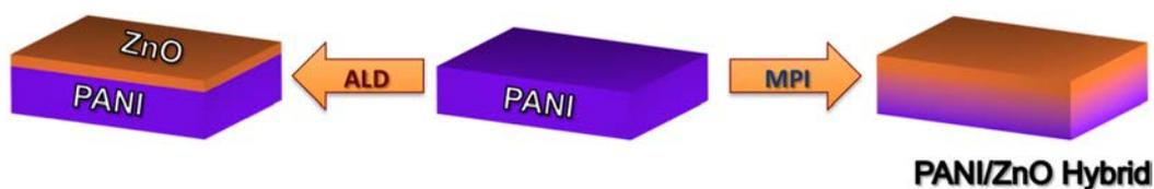
Schematic indicating the different resulting types of composites once a polymer is processed by atomic layer deposition (ALD) or multiple pulsed vapor phase infiltration (MPI).
