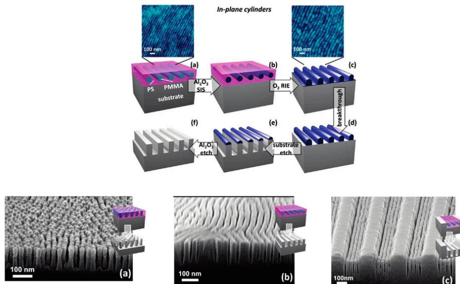
**Figure 7** Upper image: Schematics of a lithographic process. The pattern is produced from diblock-copolymers and one phase reinforced with alumina by infiltration. The remaining processing steps are common lithographic procedures. Lower image: Three examples of patterns transferred from standing PMMA cylinders, in-plane PMMA cylinders, and in-plane PMMA cylinders aligned using graphoepitaxy. Images reprinted with permission from [49]. Copyright 2011 by the American Chemical Society.
