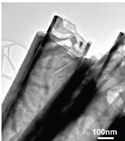
**Figure 3** Typical TEM image of  $\text{Al}_2\text{O}_3/\text{ZnO}/\text{Al}_2\text{O}_3$  microtubes (~18/10/44 nm) annealed at 700 °C for 12 h. Broken tubes clearly reveal physical separation and delineation between the inner and outer spinel tubes. The image confirms increased roughness of the spinel layers along the
