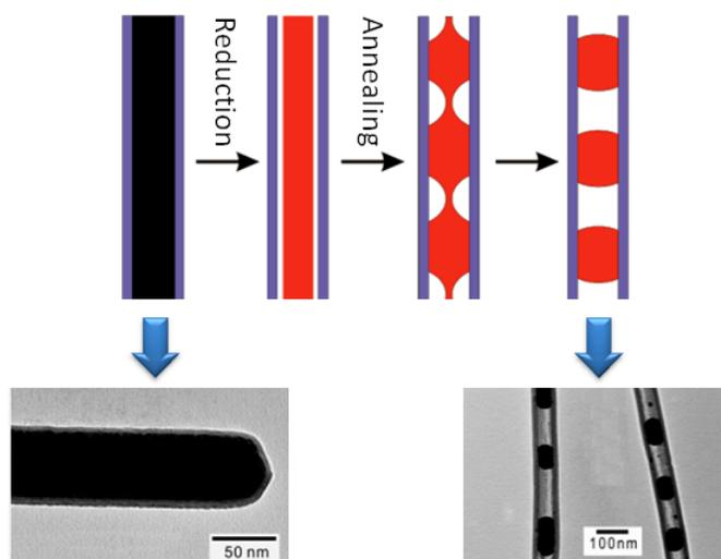
**Figure 5** Schematics of the formation process of Cu nanoparticles in metal oxide nanotubes. CuO nanowires are coated with Al<sub>2</sub>O<sub>3</sub> and subsequently reduced at elevated temperatures. The Rayleigh instability induces nanoparticle chain formation. Initial and final stages of the process are shown with typical SEM images. Figure adapted with permission from [33]. Copyright 2008 by the American Chemical Society.
