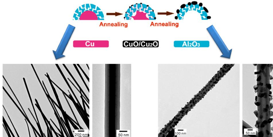
**Figure 6** Schematics of the process to produce  $\text{Cu}_x\text{O}$  nanoparticles by diffusion of Cu through an ALD coating. Initially, CuO nanowires are coated with alucone. Subsequent annealing in a  $\text{H}_2$  atmosphere
