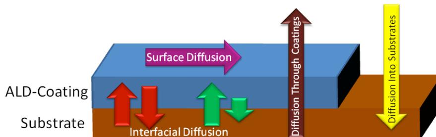
**Figure 1** Schematic overview of the various possible diffusion phenomena occurring during ALD coatings or during post-processing.
