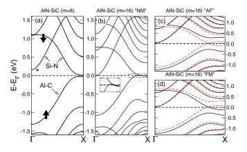
FIG. 3: (Color online) The band structure of the AlN-SiC superlattices for m=8 (a), and m=16 with paramagnetic-NM (b), antiferromagnetic-AF (c) and ferromagnetic-FM (d) solutions. Solid (black) and dashed (red) lines correspond to bands with different spin components. The inset in (b) shows the Fermi level crossing of bands at the zone boundary.
