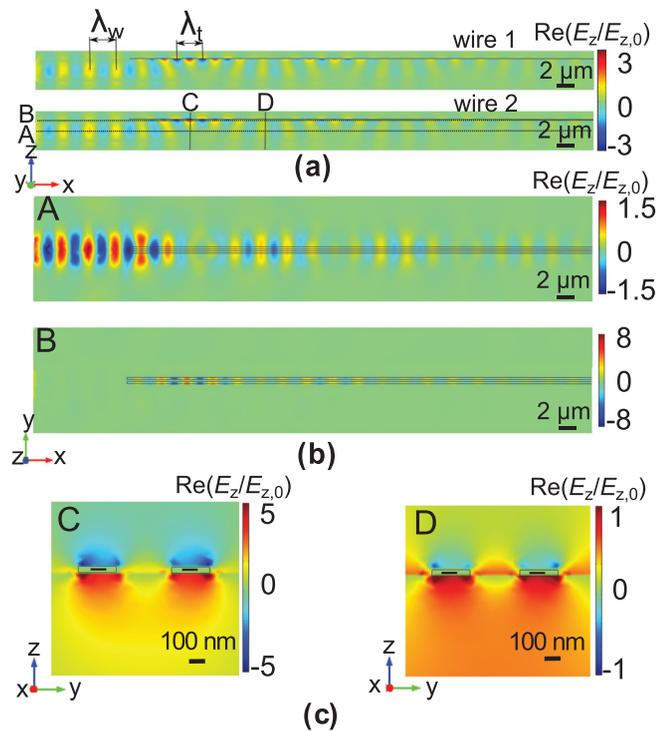
FIG. 3. Normalized real part of the electric field  $z$ -component  $\text{Re}(E_z/E_{z,0})$  obtained when exciting the hybrid structure with a wave polarized along  $z$ -direction in: (a) two  $x$ - $z$  slices at half width of each gold wire, (b)  $x$ - $y$  slices at half-height of the PhC-wg (A) and just below the TL (B); (c)  $y$ - $z$  slices at the points of maximum (C) and minimum (D) energy transfer to the TL.
