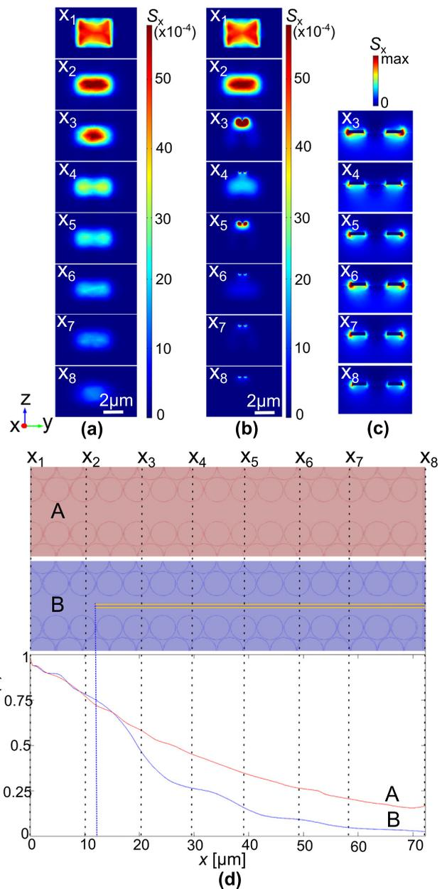
FIG. 4. Normalized Poynting vector  $S_x(x)$  along  $x$ -direction (a) without TL, (b) with the metallic TL at different  $y$ - $z$  planes ( $x_1$ - $x_8$ ), and (c) zoomed around the TL; (d) power  $P(x)$  passing through the cross section in  $x$ -direction as a function of the position  $x$  without (A) and with (B) the TL.
