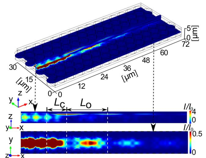
FIG. 2. Normalized electric field intensity ( $I/I_0$ ): on top, a view of the hybrid structure with  $I/I_0$  at two parallel  $x$ - $z$  planes at the center of each wire and a  $x$ - $y$  plane at the center of the silicon slab; below, individual views of one of the  $x$ - $z$  planes at the center of a wire and a subsection of the  $x$ - $y$  plane at the center of the silicon slab centered in the PhC-wg ( $L_c \approx 8 \mu\text{m}$  and  $L_o \approx 18 \mu\text{m}$ ).
