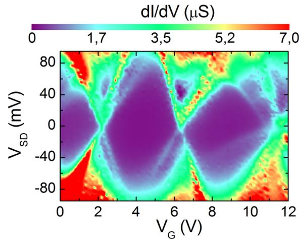
FIG. 2. Stability diagram of palladium SET obtained by electromigration. Plotting the derivative of the drain current ( $dI/dV$ ) as a function of bias voltage ( $V_{SD}$ ) and gate voltage ( $V_G$ ) results in a pattern of diamond-shaped regions of almost negligible conductance. These conductance features are a signature of the Coulomb blockade regime and they indicate the transformation of the palladium nanowires into QDs after electromigration.
