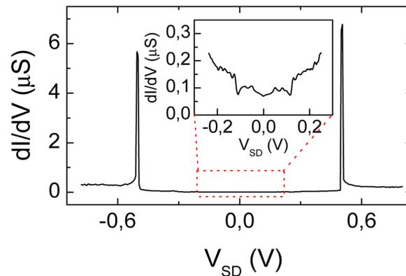
FIG. 4. Unusual conductance features in nickel devices. Sharp resonance peaks in the differential conductance curve of an electromigrated nickel device at  $T=1.8\text{K}$ . The resemblance of these features to the peaks observed in several palladium devices seems to indicate that they belong to the same type of resonance or excitation.
