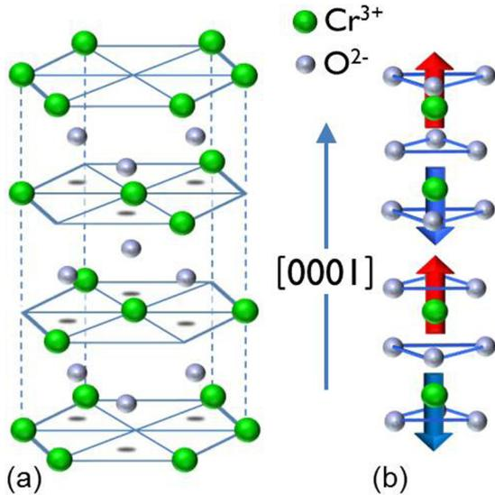
FIG. 1. (Color online) (a) Corundum crystal structure of  $\alpha$ - $\text{Cr}_2\text{O}_3$ ; (b) schematic of the antiferromagnetic (AFM) spin order. In zero magnetic field, the chromium spins are aligned antiparallel along the  $[0001]$  direction ( $c$  axis).
