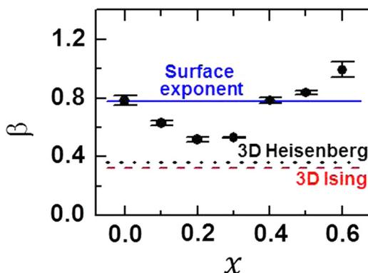
FIG. 9. (Color online)  $\text{Al}_2\text{O}_3$  concentration  $x$  dependence of the extracted critical exponent  $\beta$ . The straight (blue) line indicates the surface exponent predicted by Binder *et al.*, the (black) dotted line indicates the 3D Heisenberg model value, and the dashed (red) line shows the 3D Ising model  $\beta$  [31–33].
