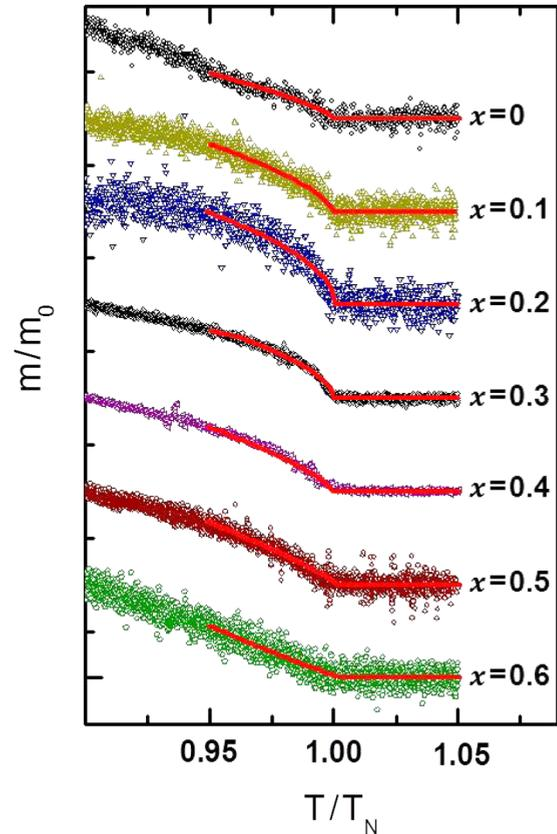
FIG. 7. (Color online) Temperature dependence of the remanent boundary magnetization in  $\text{Cr}_{2-x}\text{Al}_x\text{O}_3$  thin films of varying  $\text{Al}_2\text{O}_3$  concentration  $x$ . The (red) lines show least-squares fits to Eq. (1) for each of the sample data sets.
