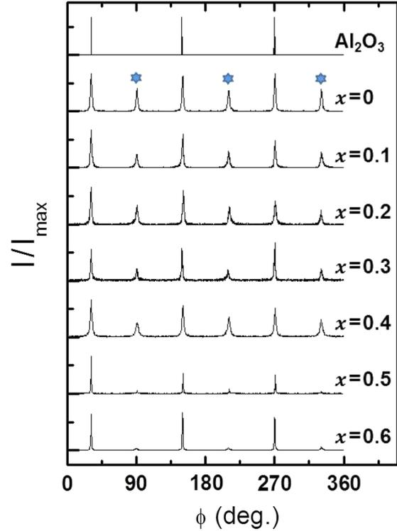
FIG. 5. (Color online) XRD  $\phi$  scans at the  $2\theta$  pole of the (10-14) planes for various  $\text{Cr}_{2-x}\text{Al}_x\text{O}_3$  thin films and for the  $\text{Al}_2\text{O}_3$  substrates. The stars mark the twinned domain positions.
