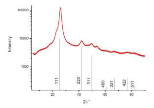
Fig. 1. X-ray Diffraction spectra of CdSe QDs. The stick pattern shows the positions of standard XRD peaks for bulk zinc blende CdSe with cubic lattice structure [18].
