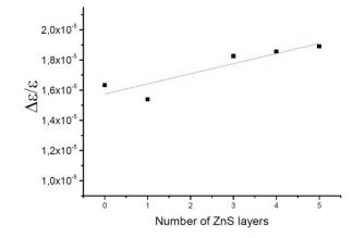
Fig. 6. Dependence of dissymmetry g-factor on the number of ZnS monolayers for CdSe QDs.
