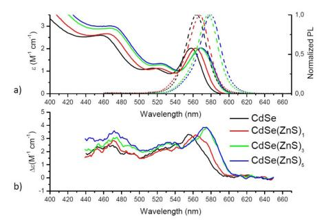
Fig. 5. a) Absorption (solid lines) and PL (dashed lines) spectra of CdSe and CdSe(ZnS) QDs (with different number of ZnS layers ranging from 1 to 5) in toluene b) CD spectra of CdSe and CdSe(ZnS)<sub>n</sub>, n = 1-5 QDs 3.4 nm size in toluene.
