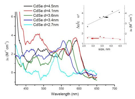
Fig. 3. CD spectra of toluene colloidal solutions of CdSe QDs of different sizes ranging from 2.7 to 4.5 nm. Inset represents the size dependence of molar CD extinction coefficient (black triangle) and g-factor of dissymmetry (red foursquare) of CdSe QDs.
