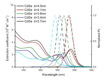
Fig. 2. Absorption (solid lines) and PL (dashed lines) spectra of toluene colloidal solutions of CdSe QDs of different sizes ranging from 2.7 to 4.5 nm solubilized with TOPO. (The PL excitation wavelength  $\lambda_{exc} = 450$  nm).
