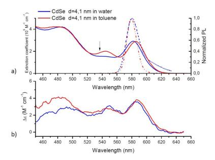
Fig. 4. a) Absorption (solid lines) and PL (dashed lines) spectra of CdSe QDs 4.1 nm size in water solution coated with DL-cysteine (blue) and in toluene coated with TOPO (red). PL excitation wavelength  $\lambda_{exc} = 450$  nm. b) CD spectra of CdSe QDs 4.1 nm size in water solution coated with DL-cysteine (blue) and in toluene coated with TOPO (red).
