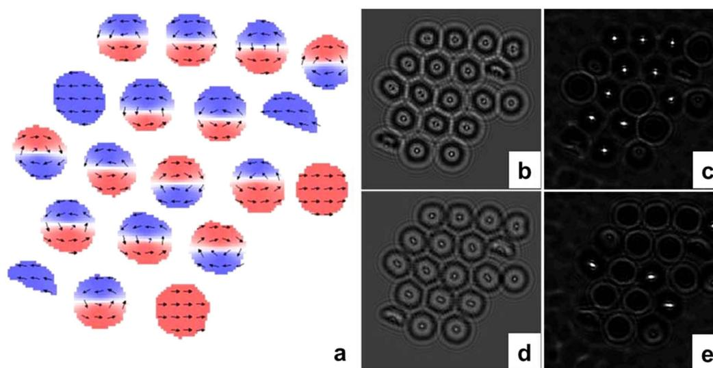
**Figure 9.** (a) The ground magnetic state on the NW array presented in the Fig. 4 (color corresponds to the magnetization component in plane with NW diameter). LorTEM images of (b,d) calculated electrostatic and (c,e) magnetic contributions. (b,c) show under- and (d,e) show over-focused images.
