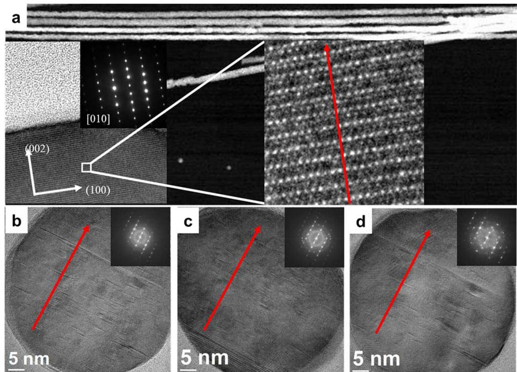
**Figure 1.** (a) Scanning TEM image of 75-nm diameter single-crystal Co NWs. In the insert the HRTEM and corresponding SAED images are shown. (b–d) HRTEM images in the plane perpendicular to the NW axis for several nanowires inside the membrane. Red arrow show the orientation of the c-axis.
