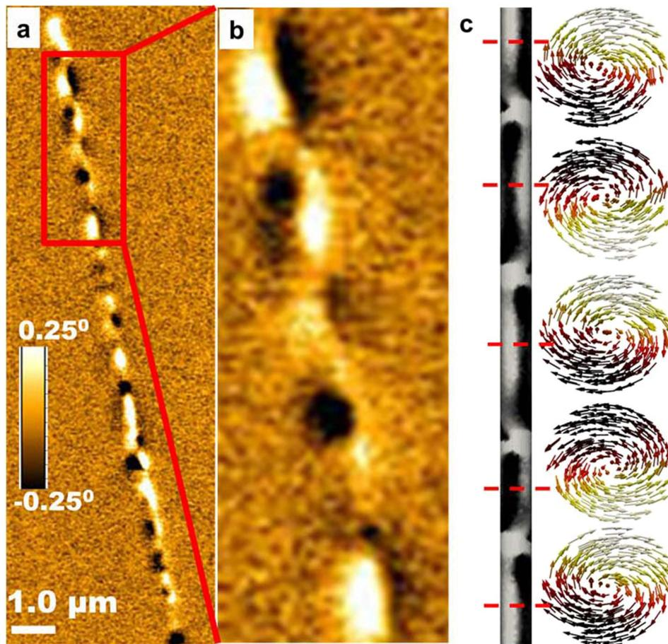
**Figure 6.** (a) A MFM image of a NW with a 45-nm diameter and a 10-μm length at remanence. (b) A close up of an area with five alternating vortices and (c) the corresponding results of a micromagnetic simulation. (The colors along the nanowire correspond to the MFM contrast obtained and the arrows show the clockwise and anticlockwise rotation of NW magnetization in adjacent vortices).
