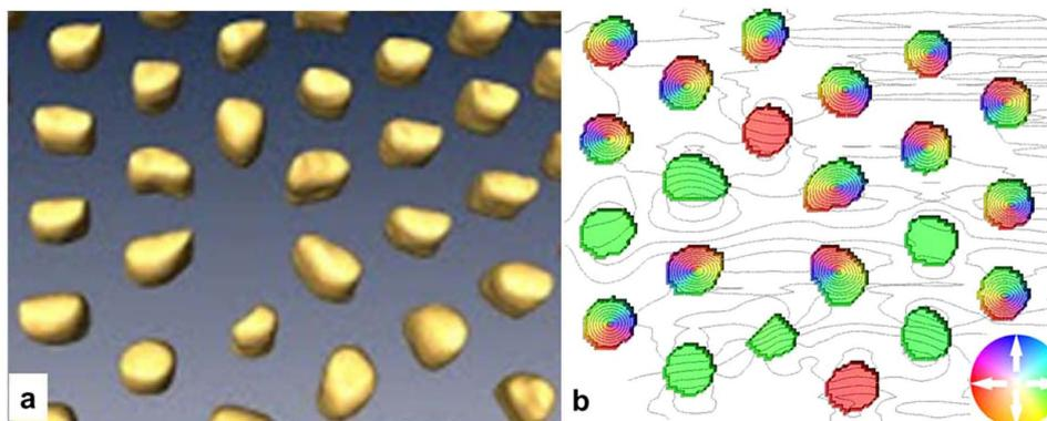
**Figure 7.** (a) A tomographic image of the section of the NW array presented in Fig. 3 and (b) the calculated ground state of magnetization (colors correspond to the in-plane component of magnetization and lines correspond to the  $B_{\perp}$ ).
