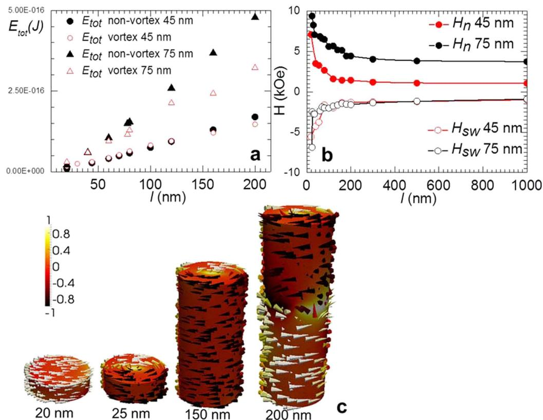
**Figure 5.** (a) Calculated dependence of the total energy of the vortex and non-vortex state on the length of NWs. (b) The nucleation field of the vortex and the switching field for the vortex core as a function of NW length after saturation in 1 T parallel to the NW axis. (c) Simulated magnetization of single-crystal hcp Co NW with a 75-nm diameter, depending on the length of the NW.
