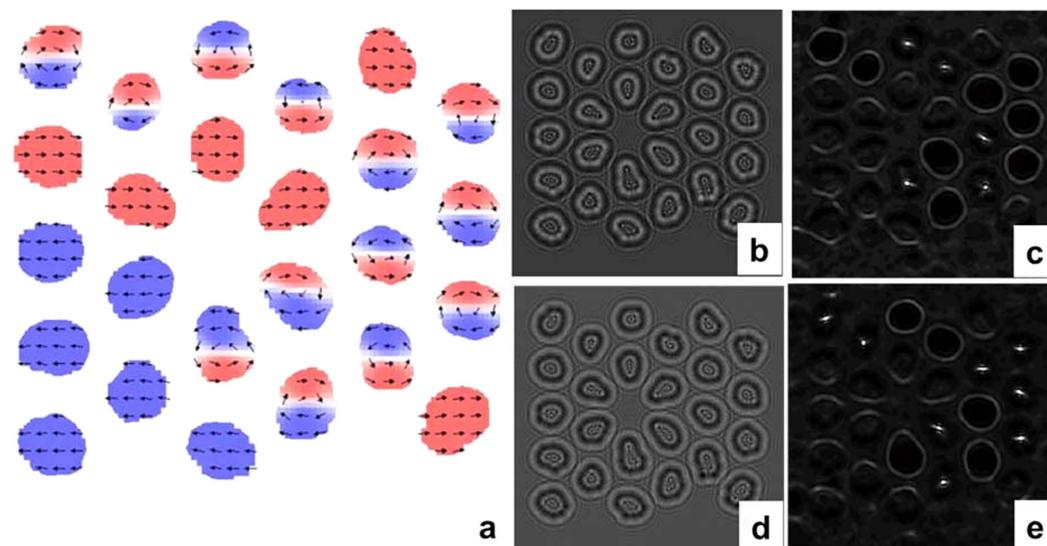
**Figure 8.** (a) The ground magnetic state on the NW array presented in Fig. 3 (color corresponds to the magnetization component in plane with NW diameter). LorTEM images of (b,d) calculated electrostatic and (c,e) magnetic contributions. (b,c) show under- and (d,e) show over-focused images.
