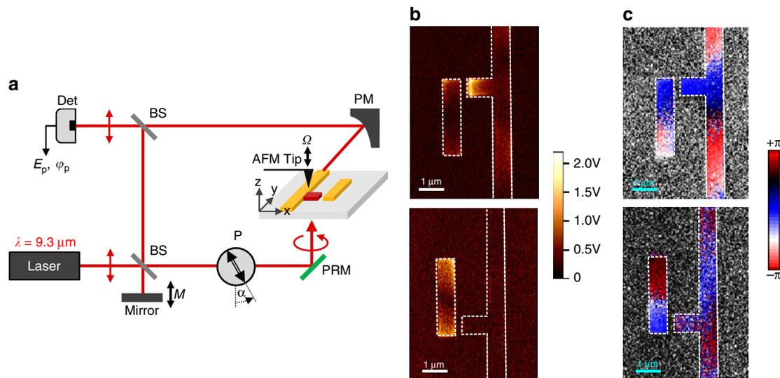
**Figure 3 | s-SNOM measurements of the optical field above two planar-chiral metasurfaces illuminated by RCP light.** (a) Schematics of the experimental setup. (b) Measured amplitude  $|E_p|$  and (c) phase of the normal electric field  $E_p$  at  $\lambda = 9.3 \mu\text{m}$ . White dashed lines in b,c outline the geometry of the structure. BS, beam splitter; Det, pseudoheterodyne detection; P, linear polarizer; PM, parabolic mirror; PRM, infrared phase retarding mirror.
