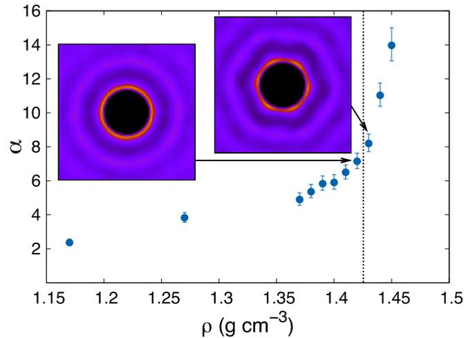
FIG. 6. Ratio between the characteristic times of  $C_{O-O}$  and  $C_{H_2O}$  at  $T = 300 \text{ K}$  with respect to density (main plot) and 2D oxygen-oxygen correlation function (insets) at  $\rho = 1.42$  (left) and  $1.43 \text{ g cm}^{-3}$  (right): the brighter the color, the larger the value of the 2D oxygen-oxygen correlation function. The vertical dashed line represents the estimated density in which the liquid-hexatic transition occurs.
