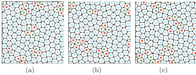
FIG. 9. [(a)–(c)] Voronoi diagram of the oxygens located in the lower layer at  $\rho = 1.47 \text{ g cm}^{-3}$ ,  $T = 300 \text{ K}$ , and three different times: (a) 0 ps, (b) 1 ps, and (c) 2 ps. Each type of polygon is marked by different colors: red (pentagon), blue (hexagon), and green (heptagon).
