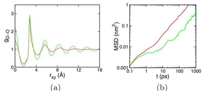
FIG. 8. (a) In-plane oxygen-oxygen radial distribution function and (b) mean-square displacement of the oxygens at  $T = 300$  K and  $\rho = 1.37$  (red) and  $1.47$  (green) g cm $^{-3}$ .
