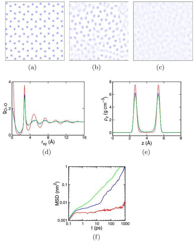
FIG. 7. [(a)–(c)] Averaged positions of the oxygens during 100 ps at  $\rho = 1.17$  g cm $^{-3}$  and three different temperatures: (a) 240 K, (b) 260 K, and (c) 280 K. (d) In-plane oxygen-oxygen radial distribution function, (e) density profile of the oxygens along the confining direction, and (f) in-plane mean-square displacement of the oxygens at  $\rho = 1.17$  g cm $^{-3}$  and three different temperatures: 240 K (red), 260 K (blue), and 280 K (green).
