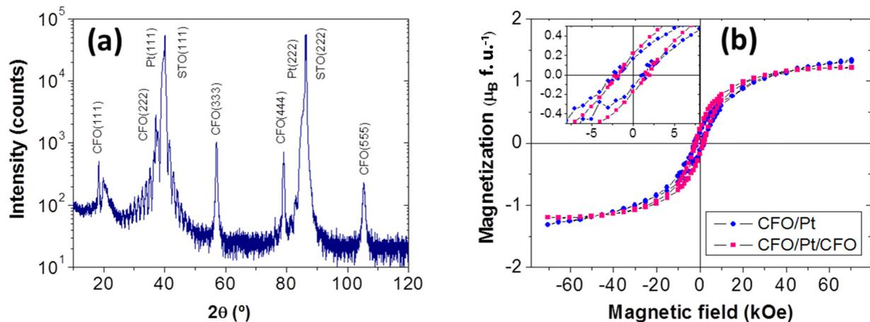
FIG. 1. (a) X-ray diffraction  $\theta$ - $2\theta$  pattern of the STO//CFO(28 nm)/Pt/CFO(28 nm) sample. (b) Room-temperature magnetization loops for the STO//CFO(28 nm)/Pt/CFO(28 nm) and STO//CFO(28 nm)/Pt samples. Inset in (b) is a zoom of the low-field region of the magnetization loops (magnetization units are Bohr magnetons per formula unit).
