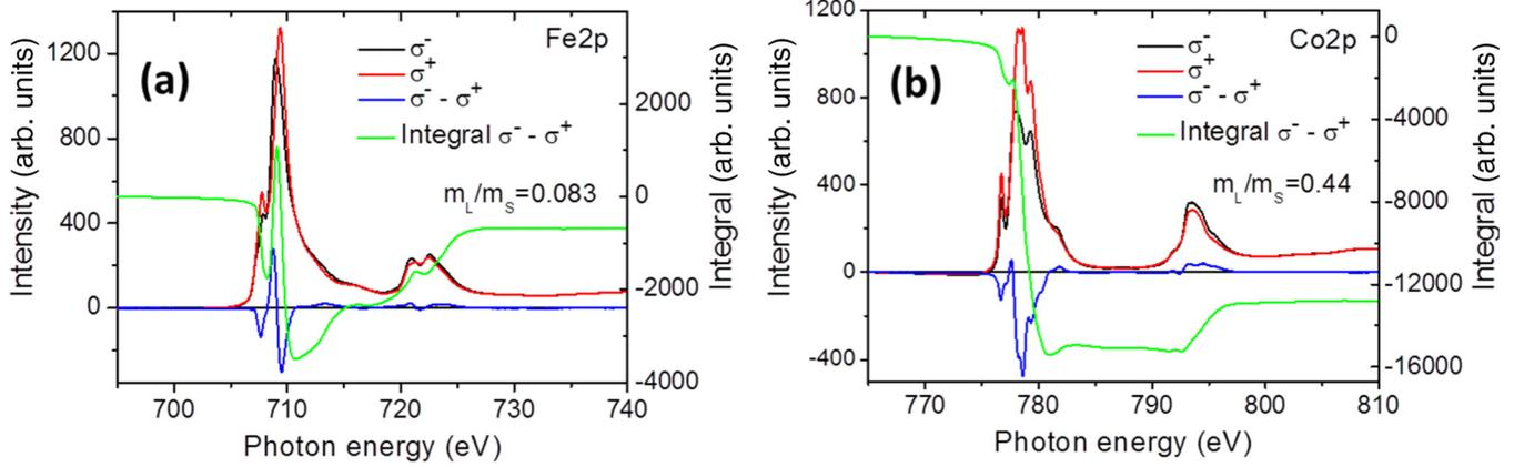
FIG. 3. (a) Fe- $L_{2,3}$  and (b) Co- $L_{2,3}$  2p XMCD spectra STO//CFO(28 nm)/Pt/CFO(28 nm) sample (295 K, 60 kOe, normal incidence). The black, red, and blue lines (left axis) show the absorption for  $\sigma^-$  and  $\sigma^+$  photon helicities and the dichroic ( $\sigma^- - \sigma^+$ ) spectra, respectively. The green line shows the integrated difference spectrum (right axis).
