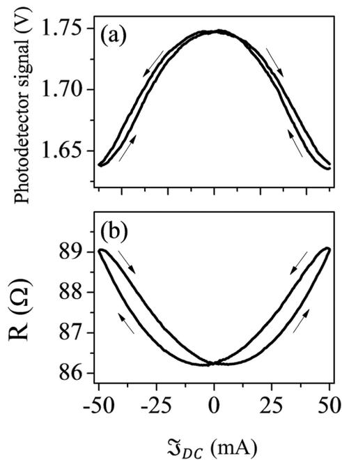
FIG. 4. Simultaneously measured (a) photodetector signal and (b) resistance as a function of the applied current, for the 15 nm Pt sample and polarizer orientations of  $\theta_1 = 90^\circ$  and  $\theta_2 = 5^\circ$ .
