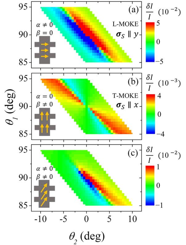
FIG. 2. Symmetry properties of  $\delta I/I(\theta_1, \theta_2)$  maps representing MOKE signals for different magnetization orientations (corresponding scale bars are shown on the right hand side in each figure): (a) Longitudinal, (b) transverse, and (c) combination of longitudinal and transverse.
