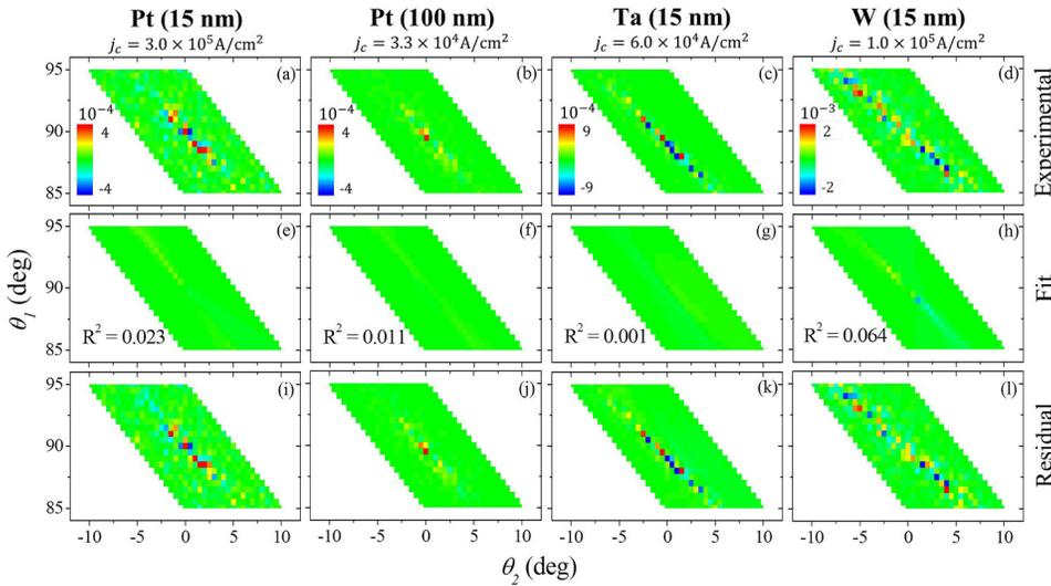
FIG. 3. (a)–(d) Experimental  $\delta I/I(\theta_1, \theta_2)$  maps for the four samples; (e)–(h) Least-squares fits of the measured maps to Eq. (3). The insets show the  $R^2$  goodness values of the fits. (i)–(l) Difference between experimental data and fits. Each column corresponds to the sample and the current density value specified on top. The scale bars for the maps corresponding to each sample are displayed inside (a)–(d), respectively.
