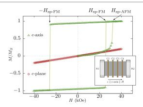
**Figure 1.** Initial magnetization curves and hysteresis loops at 2 K, for magnetic fields applied parallel (triangles) and perpendicular (diamonds) to the c-axis. The spontaneous fields for the AFM $\rightarrow$ FM transition,  $H_{\rm sp-AFM}$ , and for the FM reversal,  $\pm H_{\rm sp-FM}$ , are marked on the top axis. Inset: setup made of two resistors Ri (i=1,2), and four equidistant pick-up coils  $C_j$  (j=1,...,4); the dark-gray rectangle represents the sample.
