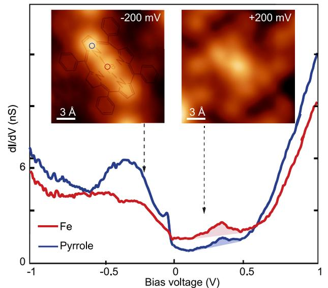
FIG. 5. Wide-range  $dI/dV$  spectra of a bright molecule measured on the locations showed in the inset ( $V_S = 1.5$  V,  $I = 3$  nA,  $V_{\text{rms}} = 2$  mV). Inset: constant-height conductance maps measured at  $V_S = -200$  mV and  $V_S = +200$  mV, respectively ( $I = 200$  pA).
