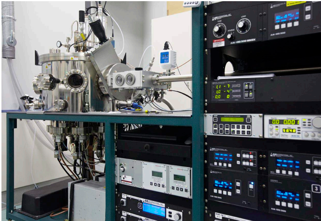
Figure 3-12: 7-gun AJA Sputtering System present at the nanomag lab in CIC nanoGUNE.
