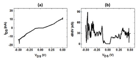
Figure 12. (a) Measurement of Coulomb staircase. Clear steps can be seen around  $V_{ds} = \pm 320 \text{mV}$ . (b) Differential conductance (dI/dV) plot of same data indicating the plateaus of conductivity
