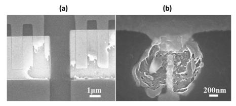
Figure 10. Device break down due to large bias. The melting of the electrodes indicated large temperatures are involved. In (b) we see that the organic material can be affected prior to the destruction of the electrodes.
