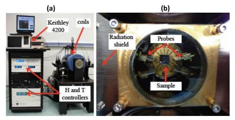
Figure 1. Probe Station Measurement Equipment. Adapted from [180]
