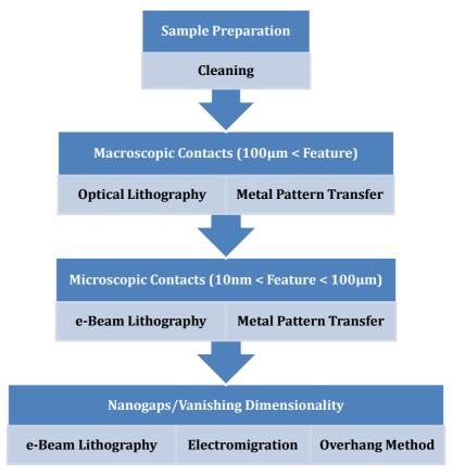
Figure 1. Flowchart of fabrication process
