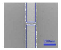
*Figure 5. SEM image of swollen EBL structures due to the proximity effect. Blue line indicates designed structure.*
