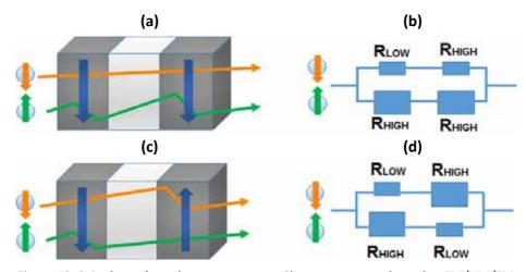
Figure 13. Spin dependent electron transport. Charge transport through a FM/NM/FM tri-layer and the equivalent circuit model for (a, b) parallel and (c, d) anti-parallel state. For most materials, the total resistance in (b) is lower than the total resistance in (d)
