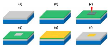
Figure 3. Work flow diagram of EBL process. (a) start with clean substrate (b) coat with resist (c) expose resist to e-beam (d) develop to remove exposed resist, creating resist window (e) deposit material (f) lift-off resist to reveal material structure
