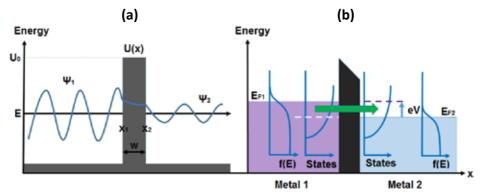
*Figure 4. (a) Electron wavefunction decays through a potential barrier and comes out on the other side. (b) Electrodes separated by and insulating barrier.*
