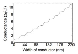
*Figure 3. Experimental observation of the quantum of conductance as observed by* [34]. *Image taken from* [35]
