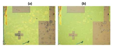
Figure 2. Optical microscope image of the effect of plasma cleaning. (a) Substrate surface covered with organic residues (b) Same substrate after soft plasma clean. After the cleaning, a considerable amount of residues has been removed.
