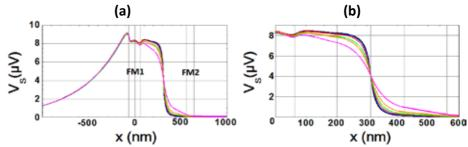
Figure 11. (a) Spin accumulation voltage due to current injection at FM1 (x=0) for different constriction sizes: 70nm (pink), 43.3nm (orange), 31.1 (green), 23.7nm (red), 18.3nm (blue) and 15.6nm(black). (b) Zoom of (a) at point of constriction.
