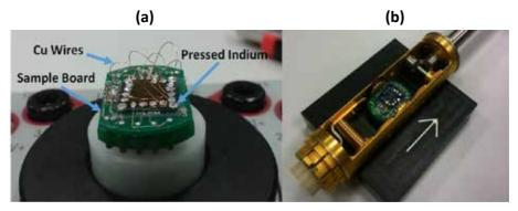
Figure 2. (a) Bonded Sample on test bed. (b) Sample in PPMS sample holder.
