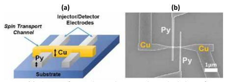
Figure 1. (a) Schematic of a Lateral Spin Valve. For our design, the thickness of Py must be substantially less than that of Cu so as to avoid discontinuity at the junction. Twoheaded black arrows indicate the thickness of the electrodes (b) SEM image of actual LSV device with constricted channel
