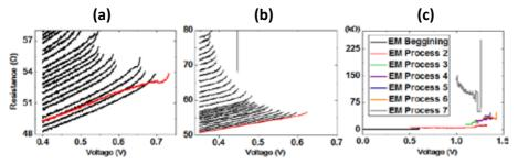
Figure 11. EM ramps of Au and Cu nanowires. (a) First EM ramp highlighted in red. (b) Controllable EM regime (c) High resistance regime.
