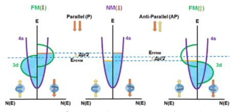
Figure 15. Detection of spin accumulation in a NM. Depending on the magnetic orientation of the detector FMs, the interfacial voltage of Vs =  $+\Delta\mu/2q$  or Vs =  $-\Delta\mu/2q$  will arise at the detector interface.
