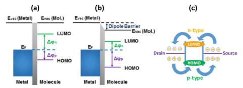
*Figure 8. (a)Metal-molecule interface without dipole (Shottky-Mott Interface [71, 72]) (b) Dipole barrier causes the trasport barriers into the LUMO and the HOMO to change. (c) n-type and p-type transport*
