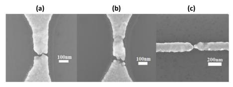
*Figure 12. EM of nanowires. (a) EM resulting in single nanogap. (b) EM resulting in two parallel conductive channels. (c) EM of wire with spatial constriction.*
