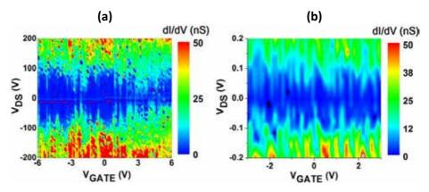
Figure 14. Stability diagrams of particles trapped during the Overhang process, displaying (a) Coulomb diamonds and (b) Coulomb shards.
