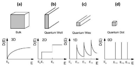
*Figure 1. Schematic diagram illustrating the representation of the electronic density of states depending on dimensionality* [7].
