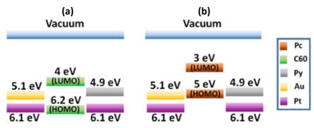
Figure 7. Rigid energy band diagram of our molecular devices with (a) C60 and (b)Pc. The metals used for source and drain electrodes were Permalloy (Py), Gold (Au) and Platinum (Pt).
