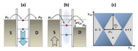
Figure 13. CB in an SET. The blockade is lifted either by applying a gate voltage  $V_G$  (a) or a source-drain voltage  $V_{SD}$  (b). (c) Sketch of a stability diagram. Light regions represent negligible conductance while darker regions represent appreciable conductance. Adapted from [204].
