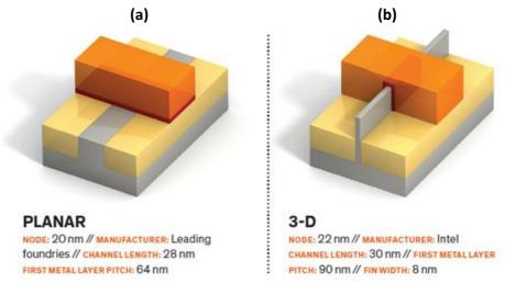
Figure 2. Manufacturers moved from the (a) planar transistor geometry to the (b) 3D transistors. Image taken from [25].
