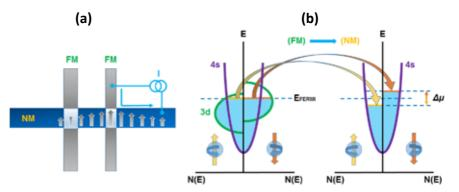
Figure 14. (a) Schematic of spin injection by means of a spin polarized current through a FM/NM interface in a LSV. The excess spins injected at the interface diffuse equilaterally throughout the NM. (b) DOS viewpoint of spin injection. The imbalance in the DOS of the FM is transferred to the NM causing each spin sub-band to shift by  $\Delta\mu/2$  from the Fermi Level.
