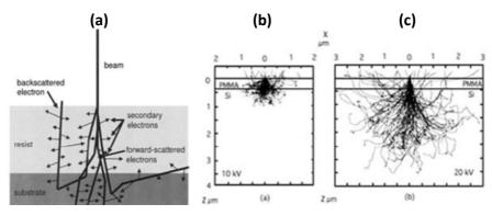
Figure 4. (a) Schematic of scattering of electrons in resist [121]. (b)Monte Carlo simulation of incoming electrons in resist for 10kV accelerating voltage and (c) 20kV accelerating voltage [122].
