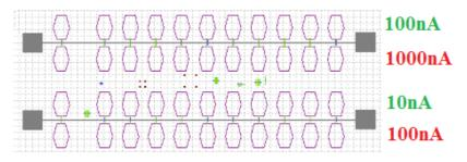
Figure 17. Design of sample fabricated using the overhang method. Current scales (for fixed bias) with the location on the substrate and the orientation of the shadow indicating large angle effects on the resulting gap size.
