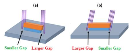
*Figure 16. (a) The substrate is tilted and not perpendicular to the incoming metal atoms. (b) The incoming atoms arrive at an angle causing the resulting shadow to increase or decrease respectively*
