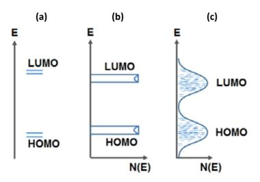
Figure 7. Energy Band diagram for  $\pi$ -conjugated (a) single molecule (b) ideal molecular crystal (c) realistic, disordered assembly of molecules. Adapted from [50].
