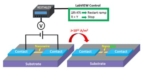
Figure 10. Schematic of EM process. A voltage source applies an increasing voltage to the nanowire in a 2-point configuration. Once the critical current density is reached EM takes place and the resistance increases abruptly. The increase in resistance resets the ramp via the feedback mechanism
