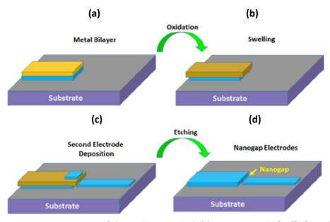
Figure 14. Process steps of the Overhang method. (a) Deposition and lift-off of metal bilayer. (b) Oxidation and swelling of top layer. (c) Second electrode is defined to overlap the bilayer. (d) Wet etching removes the top of the bilayer and the overlapping part of the second electrode exposing the nanogap.
