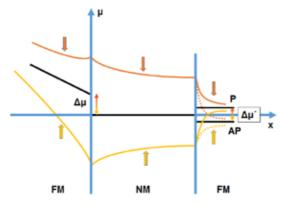
Figure 16. Schematic of the electrochemical potential for a LSV. Spins are injected at the left-most FM/NM interface creating a spin accumulation  $\Delta\mu$ . Within the NM, the spin population decays. At the second FM/NM interface spin accumulation  $\Delta\mu'$  can be detected as the difference in interfacial voltage between the parallel and anti-parallel cases.
