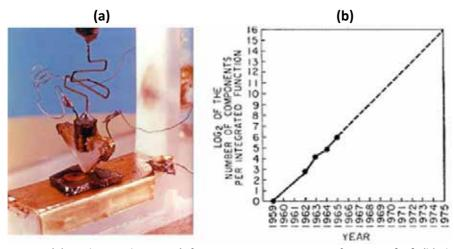
Figure 1. (a) Bardeen and Brattain's first point-contact transistor from 1947 [24]. (b) Plot from Gordon Moore's paper [22] indicating his prediction for the increase in number of electronic components per silicon chip.
