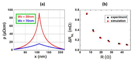
Figure 10. (a) Variation of resistivity in constricted region for 20nm constriction (red) and 70nm constriction (blue). Locally the  $\rho$  of the constriction can reach several tens of  $\mu\Omega$ cms. (b) Experimental data and simulated NL signal using  $\lambda$ =451nm and the variable  $\rho$  model described above. Agreement is very good.
