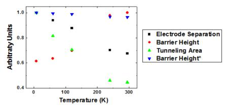
Figure 10. Normalized fitted barrier parameters for different temperature. Barrier Height\* (blue) represents that found while fixing area and separation. Barrier Height (red) represents the results of the simultaneous fit.
