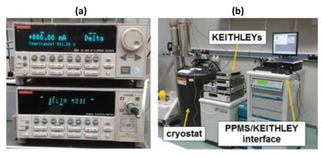
Figure 3. (a) 6221 Current Source (top) and 2182 nanovoltmeter (bottom) coupled for delta mode measurements. (b) Entire set-up. Cryostat, Switchbaord, KEITHLEYs and computer interface.
