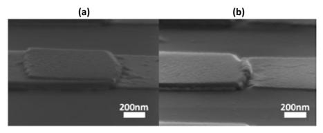
Figure 15. Bilayer (left) and overlapping electrode (right) before etching. (a)Large Overlap. (b)Small Overlap.
