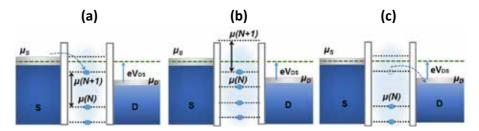
Figure 10. Applying  $V_{DS}$  lifts CB. (a)Tunneling from source electrode to dot. (b)Addition of electron raises the energy of the dot by  $E_{Add}$ .(c) Electron Tunnels off the dot and into the drain electrode. Images adapted from [73].
