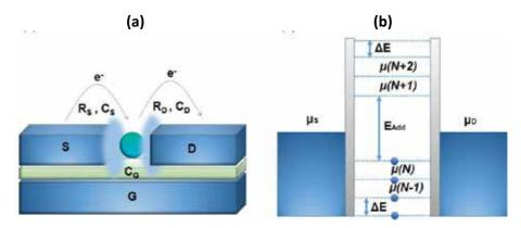
Figure 9. (a)Single Electron Transistor (SET). R represents the tunnel resistance of the barriers around the island, C is the capacitance and S,D and G represent source drain and gate electrodes respectively (b) Energy landscape of SET, adapted from [73]
