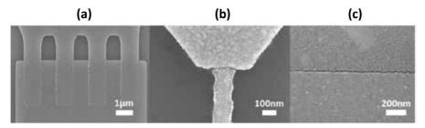
*Figure 19. Devices made using Overhang Method. (a) Interdigitated electrodes (b) Low aspect ratio electrodes (c) Large aspect ratio electrodes*
