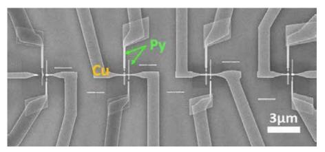
Figure 2. SEM image taken after the measurement process showing undesirable EM of the LSVs' FM electrodes.
