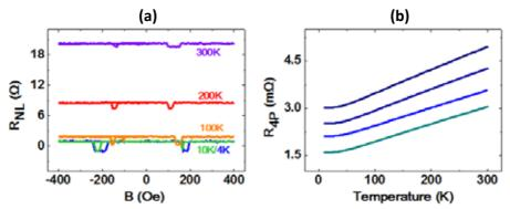
Figure 5. (a) NL signal at different temperatures. The  $\Delta R_{NL}$  values are 0.6m $\Omega$  (300K), 1.08m $\Omega$  (200K), 1.55m $\Omega$  (100K) and 1.76m $\Omega$  (10K/4K) showing a clear increase of spin signals at low temperatures. (b) Channel resistance (4-point) between 10K and 300K for four distinct samples. The Cu resistivity decreases with temperature and saturates around 10K.
