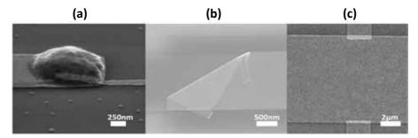
Figure 18. Failed lift-off. (a)Residues of the etch left under the overlapping metal. The edges did not allow the excess metal to rip off. (b) Excess metal ripping off in interdigitated design. The large border requires a large amount of ripping which impedes the removal of excess material. (c) Failed lift-off. Excess material is removed but rip occurred over bilayer.
