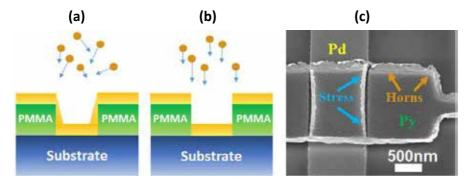
Figure 8. (a) Omni-directional deposition. Material is deposited on side-walls of resist. (b)Directional deposition. Material is deposited only in desired location. (c) SEM image of e-beam (directional) deposited Py structure with horns. (a) and (b) adapted from [125].
