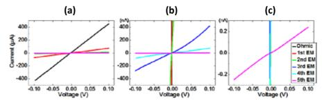
Figure 13. I(V) curves at various EM steps. During EM we see the transition from Ohmic (a) to non-linear (c) behavior.
