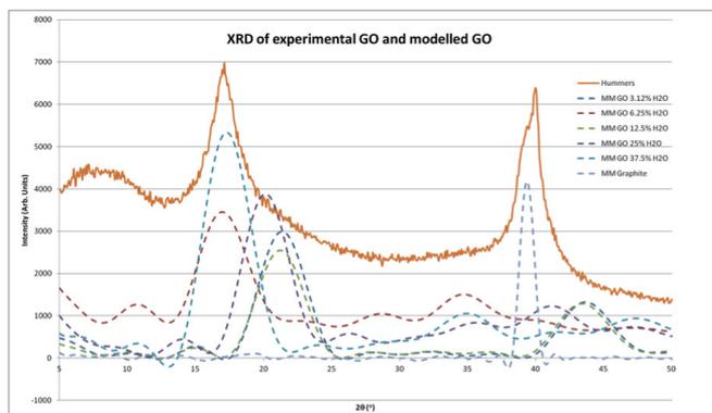
Figure 1. XRD Experimental and simulated patterns of graphite oxide.
