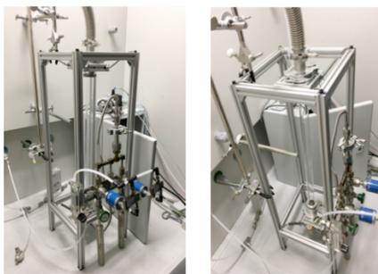
Figure. The fluidized bed reactor (FBR) configuration for coating nanoparticles using ALD.
